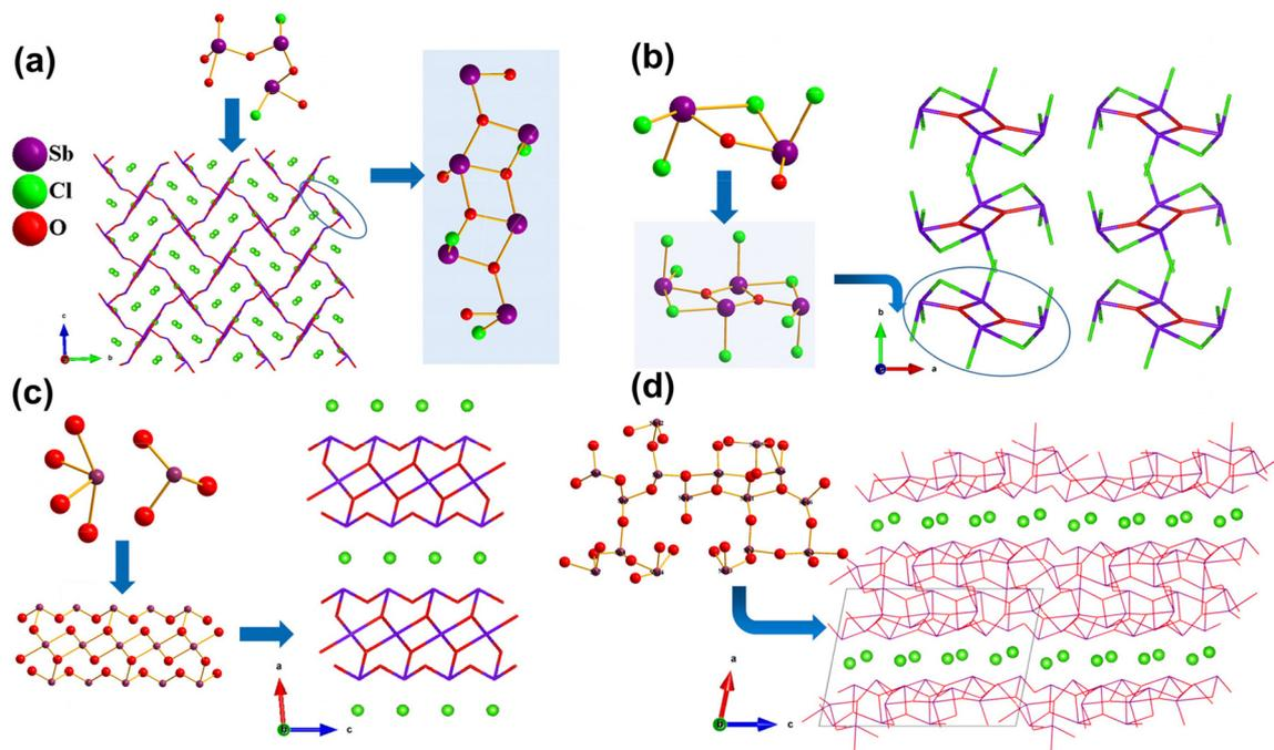
**Fig. 2** Crystals structure information about compounds studied in this work. (a) The structure of  $\text{SbOCl}$  along the  $a$  axis; (b) the structure of  $\text{Sb}_2\text{OCl}_4$  along the  $c$  axis; (c) the structure of  $\text{Sb}_3\text{O}_4\text{Cl}$  along the  $b$  axis; (d) the structure of  $\text{Sb}_8\text{O}_{11}\text{Cl}_2$  along the  $c$  axis.
