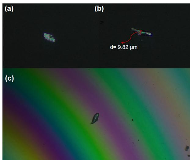
**Fig. 3** Birefringence measurements for the  $\text{Sb}_2\text{OCl}_4$  crystals. (a) Original interference color of the  $\text{Sb}_2\text{OCl}_4$  crystal under orthogonally polarized light. (b) The thickness view of  $\text{Sb}_2\text{OCl}_4$  crystal. (c) Extinction of the measurement of refractive index difference.
