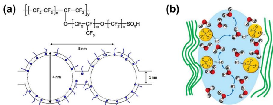
**Fig. 5** (a) Structure of Nafion and the cluster-network model. Hydrophilic clusters are connected by short narrow channels. Short curves represent Nafion side chains and dots represent sulfonic acid groups. Reproduced from ref. 84 with permission from Elsevier, Copyright 1983. (b) Proton conduction mechanism in hydrophilic region of hydrated proton exchange membrane. Reproduced from ref. 87 with permission from John Wiley and Sons, Copyright 2023.
