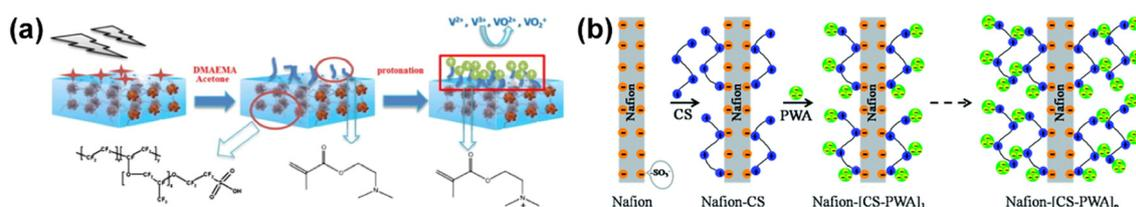
**Fig. 9** (a) Preparation of radiation-induced grafted Nafion-*g*-PDMAEMA and protonated Nafion-*g*-PDMAEMA. Reproduced from ref. 100 with permission from Elsevier, Copyright 2013. (b) Schematic diagram of layer-by-layer self-assembly of Nafion-[CS-PWA]<sub>*n*</sub> membrane. Reproduced from ref. 50 with permission from The Royal Society of Chemistry, Copyright 2014.
