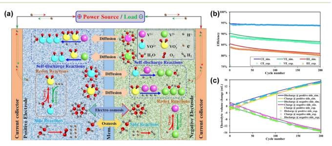
Fig. 4 (a) Illustration of chemical reactions, species crossover and water transport in VRFB. (b) Comparison of the coulombic efficiency, voltage efficiency and energy efficiency of VRFB. (c) Simulation and experimental results of electrolyte volume changes in the catholyte and anolyte tanks after each cycle. Reproduced from ref. 80 with permission from Elsevier, Copyright 2023.
