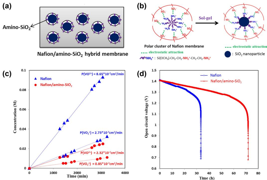
**Fig. 6** (a) Schematic illustration of Nafion/inorganic hybrid membrane. (b) Preparation of Nafion/amino-SiO<sub>2</sub> hybrid membrane. (c) Effect of Nafion and Nafion/amino-SiO<sub>2</sub> membrane on intracellular VO<sup>2+</sup> and VO<sub>2</sub><sup>+</sup> concentration. (d) OCV of VRFB over time using Nafion and Nafion/amino-SiO<sub>2</sub> membrane in the charged state of 75%. Reproduced from ref. 92 with permission from Elsevier, Copyright 2015.
