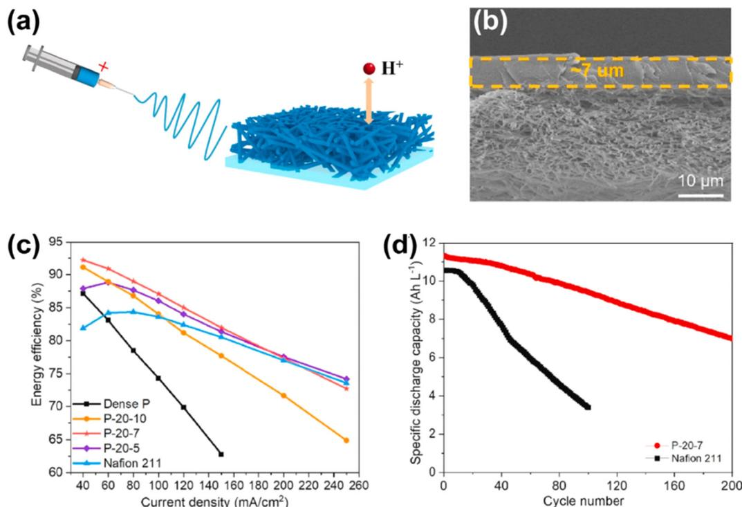
**Fig. 13** (a) Illustrative scheme of PBI composite membrane supported by electrospun nanofibers. (b) SEM images of the cross-section morphology of P-20-7. (c) Energy efficiency of flow batteries assembled with PBI-based membranes and Nafion 211. (d) Specific discharge capacity of flow batteries assembled with P-20-7 membrane and Nafion 211 at a current density of 80 mA cm<sup>-2</sup>. Reproduced from ref. 148 with permission from Elsevier, Copyright 2021.
