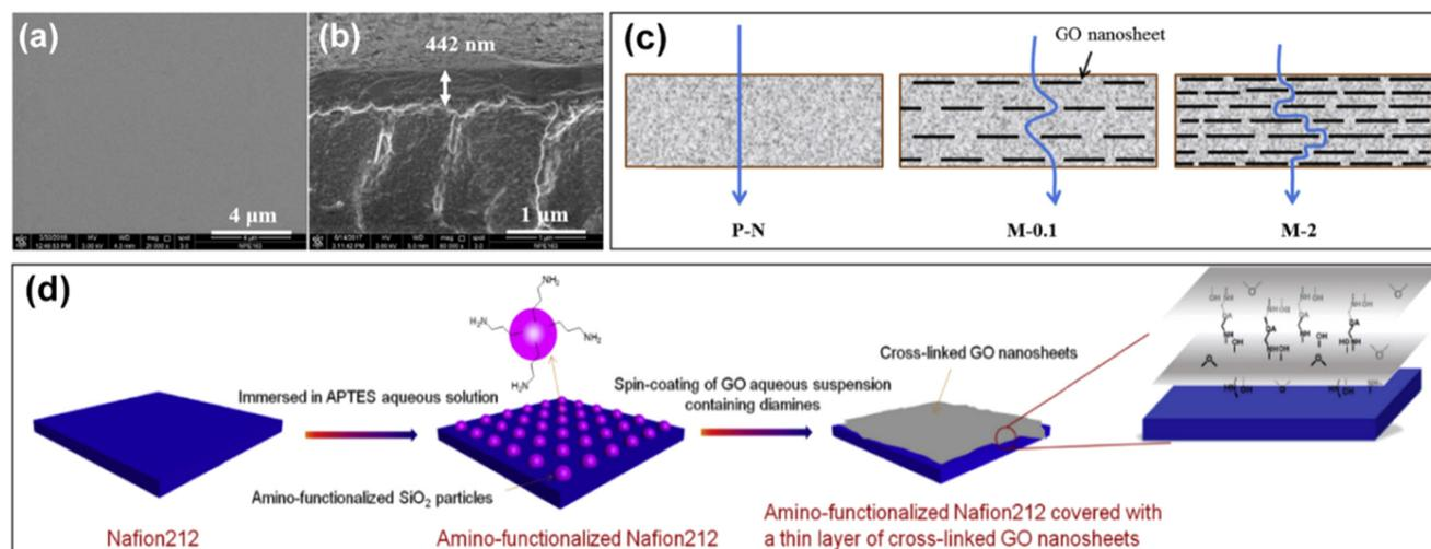
**Fig. 8** SEM images of (a) surface and (b) cross-section of graphene oxide/Nafion membrane. (c) Schematic diagram of permeation of vanadium ions in pure Nafion and graphene oxide/Nafion composite membrane. Reproduced from ref. 55 with permission from Elsevier, Copyright 2017. (d) Process for the preparation of amino-functionalized Nafion212 covered with graphene oxide nanosheets. Reproduced from ref. 98 with permission from Elsevier, Copyright 2019.
