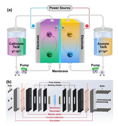
Fig. 1 Schematic diagram of (a) a vanadium redox flow battery (VRFB) system and (b) single cell.
