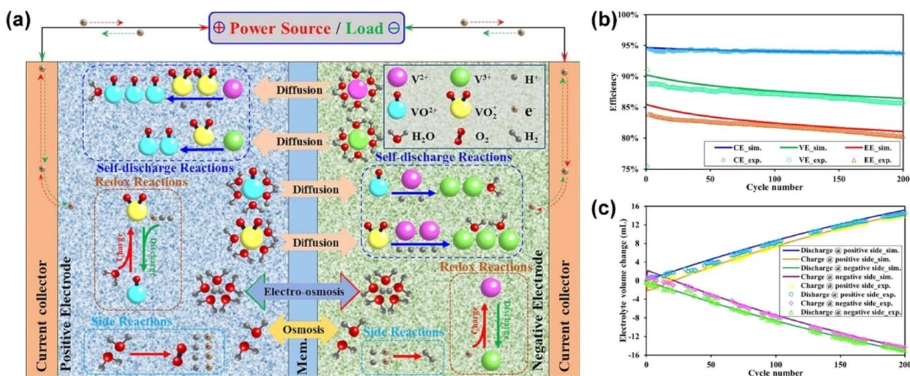
**Fig. 4** (a) Illustration of chemical reactions, species crossover and water transport in VRFB. (b) Comparison of the coulombic efficiency, voltage efficiency and energy efficiency of VRFB. (c) Simulation and experimental results of electrolyte volume changes in the catholyte and anolyte tanks after each cycle. Reproduced from ref. 80 with permission from Elsevier, Copyright 2023.
