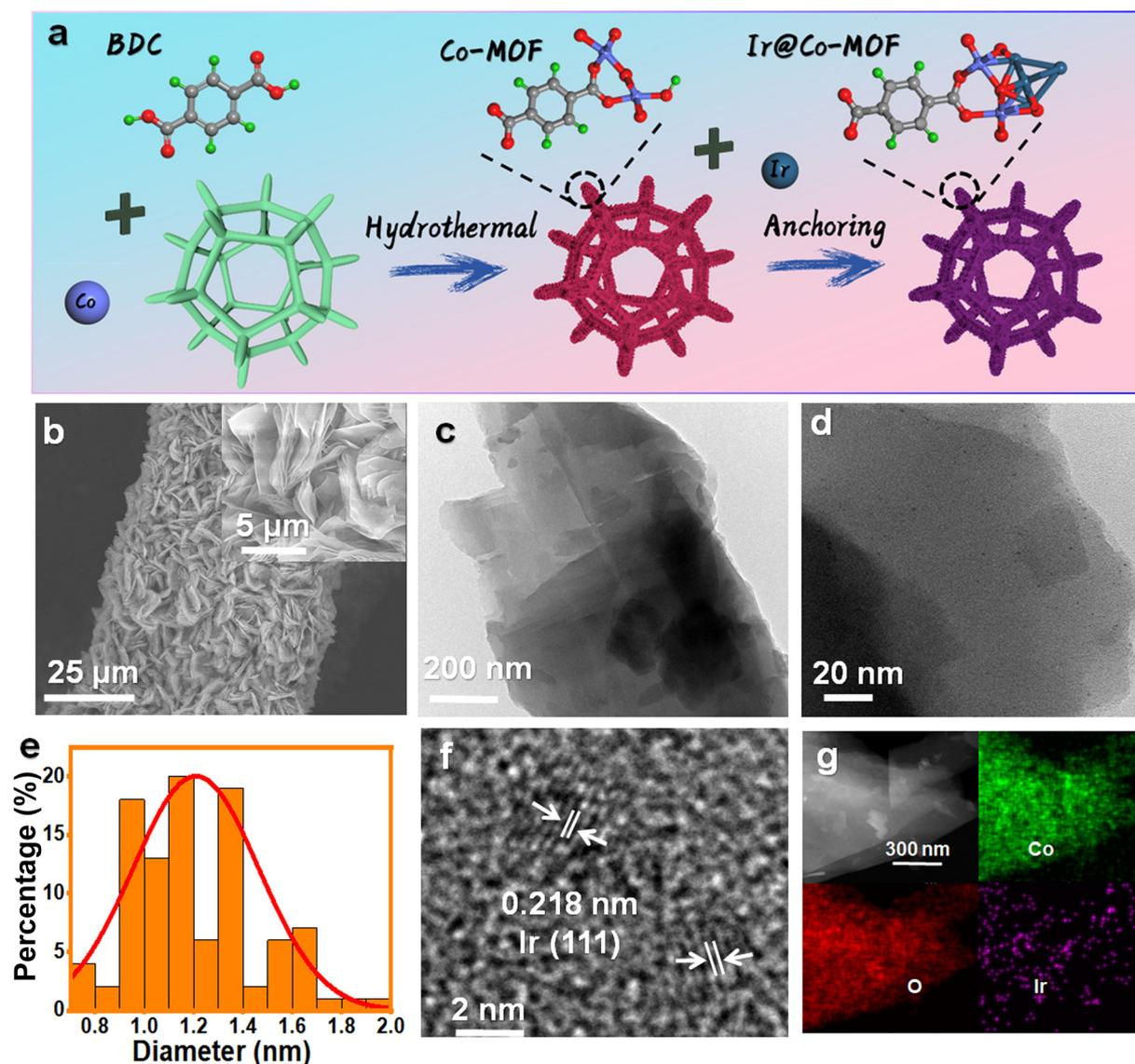
**Fig. 1** (a) Schematic illustration of the synthesis of Ir@Co-MOF. (b) images of Ir@Co-MOF. (c and d) TEM images at different magnifications of Ir@Co-MOF. (e) The size distribution of Ir nanoparticles. (f) HRTEM and (g) EDS mappings of Ir@Co-MOF.
