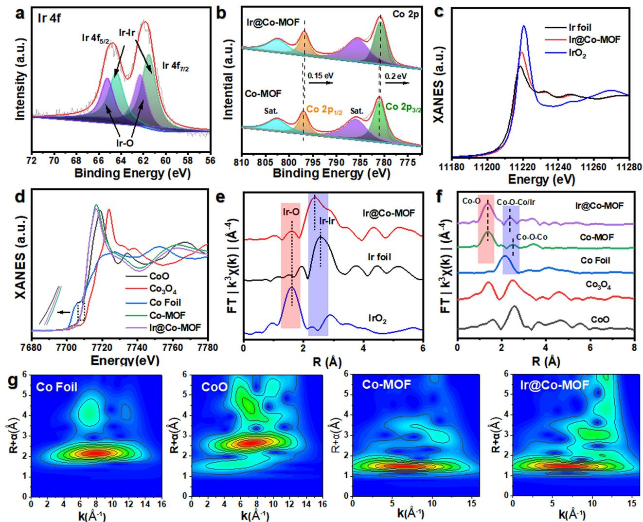
Fig. 2 XPS spectra of prepare samples. (a) Ir 4f, (b) Co 2p, of Ir@Co-MOF and Co-MOF. (c and d) The normalized XANES spectra (e and f) FT-EXAFS spectra and (g) Wavelet transform for  $k^3$ -weighted EXAFS signal of Ir foil, IrO<sub>2</sub>, Co Foil, CoO, Co-MOF and Ir@Co-MOF, respectively.
