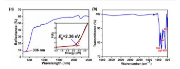
Fig. 3 (a) UV-Vis-NIR diffuse reflectance and absorption spectra of NaVSeO<sub>5</sub>; (b) IR spectrum of NaVSeO<sub>5</sub>.
