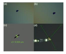
Fig. 4 (a and b) Extinction views of the crystal by negative and positive rotational compensators; (c) view of the crystal thickness; (d) orientation of the NaVSeO<sub>5</sub> crystal determined by X-ray single-crystal diffraction.
