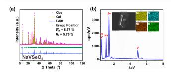
Fig. 1 (a) Rietveld refinement of the powder X-ray diffraction pattern of compound NaVSeO<sub>5</sub> polycrystals. A full Rietveld refinement was carried out using GSAS II software. (b) EDS maps of Na, V, Se, and O in the compound crystal. Scale bar is 2.5 μm.
