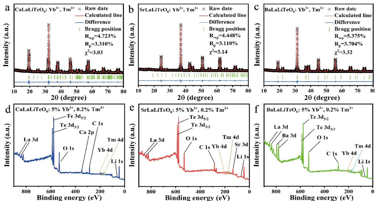
Fig. 2 XRD refined picture of (a) CaLaLiTeO<sub>6</sub>:5%Yb<sup>3+</sup>,0.2%Tm<sup>3+</sup>, (b) SrLaLiTeO<sub>6</sub>:5%Yb<sup>3+</sup>,0.2%Tm<sup>3+</sup>, and (c) BaLaLiTeO<sub>6</sub>:5%Yb<sup>3+</sup>,0.2%Tm<sup>3+</sup>. XPS spectra of (d) CaLaLiTeO<sub>6</sub>:5%Yb<sup>3+</sup>,0.2%Tm<sup>3+</sup>, (e) SrLaLiTeO<sub>6</sub>:5%Yb<sup>3+</sup>,0.2%Tm<sup>3+</sup>, and (f) BaLaLiTeO<sub>6</sub>:5%Yb<sup>3+</sup>,0.2%Tm<sup>3+</sup>.
