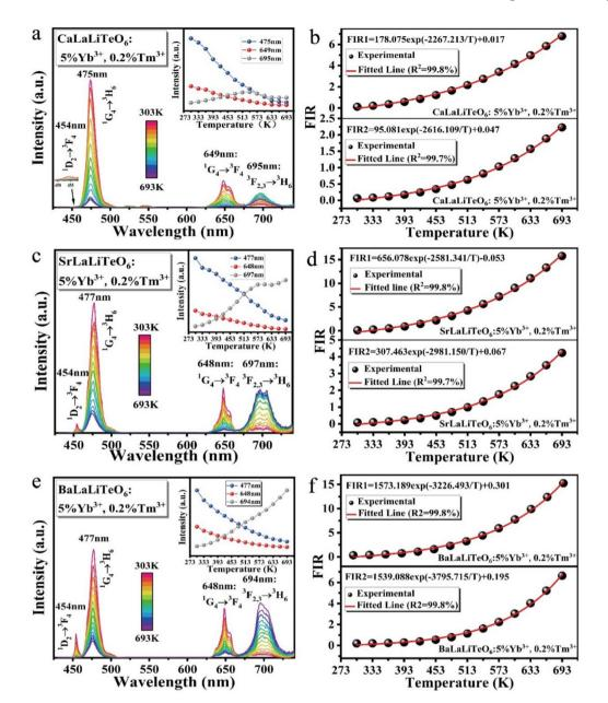
Fig. 6 (a, c and e) The temperature-dependent PL spectra of ALaLiTeO<sub>6</sub>:5%Yb<sup>3+</sup>,0.2%Tm<sup>3+</sup> phosphors (inset: the PL emission intensity versus various temperatures). (b, d and f) The calculated temperature-dependent fluorescence intensity ratios of FIR<sub>1</sub> = ( ${}^{3}F_{2,3} \rightarrow {}^{3}H_{6}$ )/( ${}^{1}G_{4} \rightarrow {}^{3}F_{4}$ ) and FIR<sub>2</sub> =  $({}^{3}F_{2,3} \rightarrow {}^{3}H_{6})/({}^{1}G_{4} \rightarrow {}^{3}H_{6}).$
