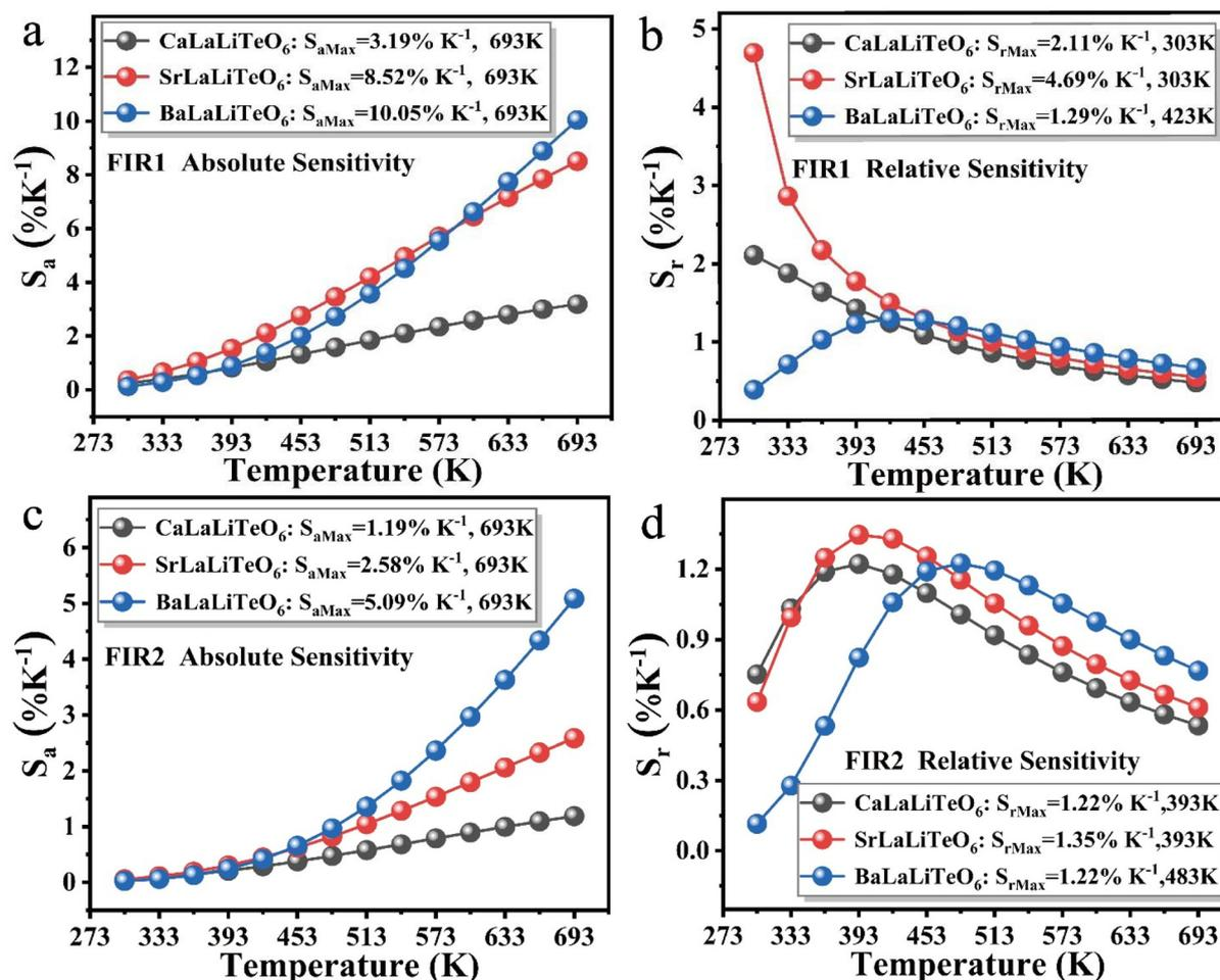
Fig. 7 (a and b) The calculated  $S_a$  and  $S_r$  values of  $\text{ALaLiTeO}_6:\text{Yb}^{3+},\text{Tm}^{3+}$  based on  $\text{FIR}_1$ . (c and d) The calculated  $S_a$  and  $S_r$  values of  $\text{ALaLiTeO}_6:\text{Yb}^{3+},\text{Tm}^{3+}$  based on  $\text{FIR}_2$ .
