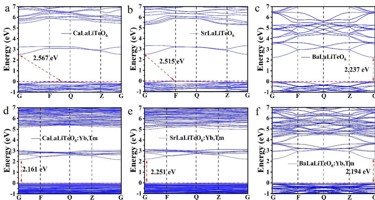
Fig. 4 Calculated band structures of (a–c)  $ALiTeO_6$  and (d–f)  $ALiTeO_6:Yb,Tm$  with ( $A = Ca, Sr, \text{ and } Ba$ ).
