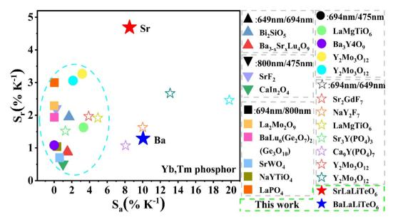
Fig. 8 Comparison of thermometry sensitivity between ALaLiTeO<sub>6</sub>:5%Yb<sup>3+</sup>,0.2%Tm<sup>3+</sup> and other Yb<sup>3+</sup> and Tm<sup>3+</sup> co-doped phosphors.
