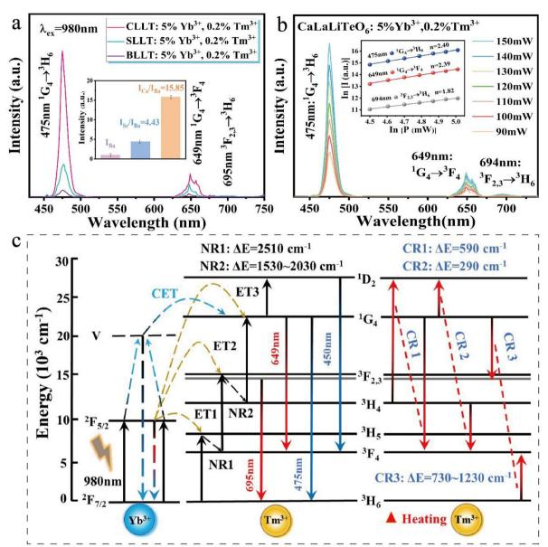
Fig. 3 (a) Up-conversion PL spectra of ALaLiTeO<sub>6</sub>:5%Yb<sup>3+</sup>,0.2%Tm<sup>3+</sup> (A = Ca, Sr, and Ba). (b) The relationship between ln(i) and ln(P) of CalaLiTeO<sub>6</sub>:5%Yb<sup>3+</sup>,0.2%Tm<sup>3+</sup>. (c) Energy level diagram and thermally enhanced CR processes in the AlaLiTeO<sub>6</sub>:5%Yb<sup>3+</sup>,0.2%Tm<sup>3+</sup> phosphor.
