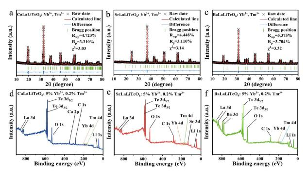
Fig. 2 XRD refined picture of (a) CalaLiTeO<sub>6</sub>:5%Yb<sup>3+</sup>,0.2%Tm<sup>3+</sup>, (b) SrLaLiTeO<sub>6</sub>:5%Yb<sup>3+</sup>,0.2%Tm<sup>3+</sup>, and (c) BalaLiTeO<sub>6</sub>:5%Yb<sup>3+</sup>,0.2%Tm<sup>3+</sup>. XPS spectra of (d) CaLaLiTeO<sub>6</sub>:5%Yb<sup>3+</sup>,0.2%Tm<sup>3+</sup>, (e) SrLaLiTeO<sub>6</sub>:5%Yb<sup>3+</sup>,0.2%Tm<sup>3+</sup>, and (f) BaLaLiTeO<sub>6</sub>:5%Yb<sup>3+</sup>,0.2%Tm<sup>3+</sup>.
