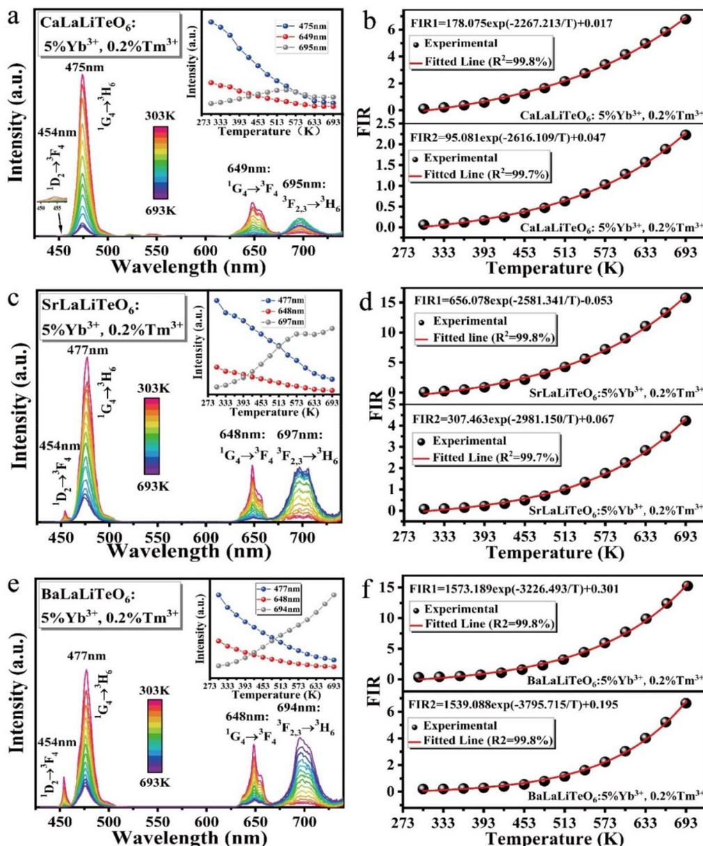
Fig. 6 (a, c and e) The temperature-dependent PL spectra of AlLaLiTeO<sub>6</sub>:5%Yb<sup>3+</sup>,0.2%Tm<sup>3+</sup> phosphors (inset: the PL emission intensity versus various temperatures). (b, d and f) The calculated temperature-dependent fluorescence intensity ratios of FIR<sub>1</sub> = (I<sub>649</sub> → I<sub>475</sub>) and FIR<sub>2</sub> = (I<sub>695</sub> → I<sub>475</sub>).
