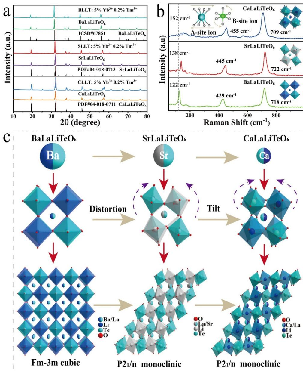
**Fig. 1** (a) XRD patterns of the non-doped and 5% Yb<sup>3+</sup>, 0.2% Tm<sup>3+</sup> co-doped ALiTeO<sub>6</sub> (A = Ca, Sr and Ba). (b) Raman spectra and (c) crystal structure of ALiTeO<sub>6</sub> (A = Ca, Sr and Ba).
