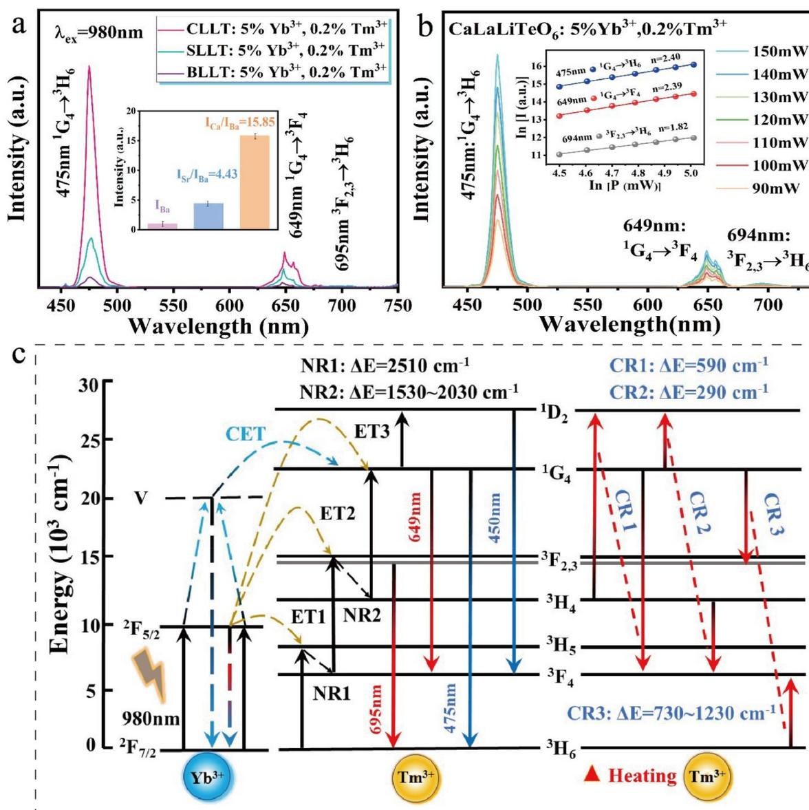
Fig. 3 (a) Up-conversion PL spectra of  $\text{ALaLiTeO}_6:5\% \text{Yb}^{3+}, 0.2\% \text{Tm}^{3+}$  (A = Ca, Sr, and Ba). (b) The relationship between  $\ln(I)$  and  $\ln(P)$  of  $\text{CaLaLiTeO}_6:5\% \text{Yb}^{3+}, 0.2\% \text{Tm}^{3+}$ . (c) Energy level diagram and thermally enhanced CR processes in the  $\text{ALaLiTeO}_6:5\% \text{Yb}^{3+}, 0.2\% \text{Tm}^{3+}$  phosphor.
