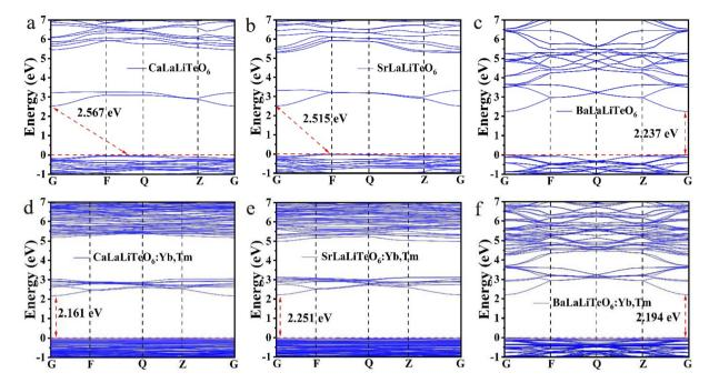
Fig. 4 Calculated band structures of (a-c) ALaLiTeO<sub>6</sub> and (d-f) ALaLiTeO<sub>6</sub>:Yb,Tm with (A = Ca, Sr, and Ba).
