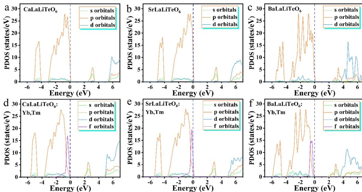
Fig. 5 The PDOS, bonding and anti-bonding orbitals of (a–c)  $\text{AlLaLiTeO}_6$  and (d–f)  $\text{AlLaLiTeO}_6:\text{Yb,Tm}$  with (A = Ca, Sr, and Ba).
