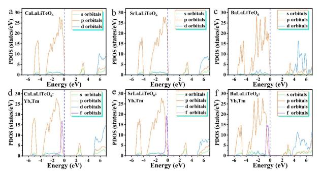
Fig. 5 The PDOS, bonding and anti-bonding orbitals of (a-c) ALaLiTeO<sub>6</sub> and (d-f) ALaLiTeO<sub>6</sub>:Yb,Tm with (A = Ca, Sr, and Ba).
