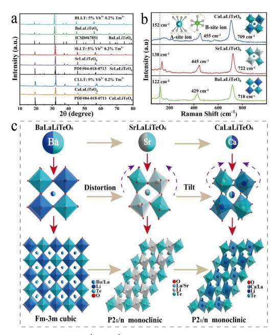
Fig. 1 (a) XRD patterns of the non-doped and 5% Yb3+, 0.2% Tm3+ co-doped ALaLiTeO<sub>6</sub> (A = Ca, Sr and Ba). (b) Raman spectra and (c) crystal structure of ALaLiTeO<sub>6</sub> (A = Ca, Sr and Ba).
