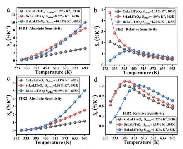
Fig. 7 (a and b) The calculated  $S_a$  and  $S_r$  values of ALaLiTeO<sub>6</sub>:Yb<sup>3+</sup>,Tm<sup>3+</sup> based on FIR<sub>1</sub>. (c and d) The calculated  $S_a$  and  $S_r$  values of ALaLiTeO<sub>6</sub>:Yb<sup>3+</sup>, Tm<sup>3+</sup> based on FIR<sub>2</sub>.
