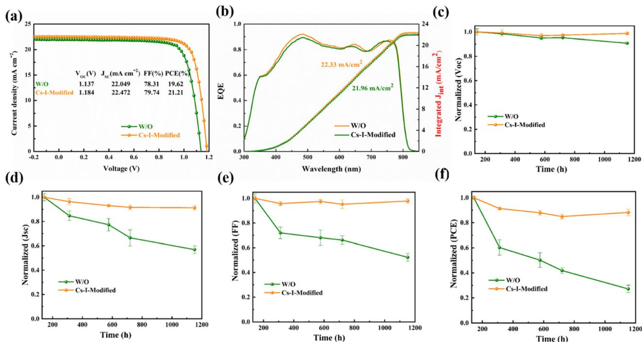
**Fig. 6** (a) Comparison of  $J$ - $V$  curves of the champion devices and their (b) EQE and corresponding integrated  $J_{int}$  curves. The stability comparison of (c)  $V_{oc}$ , (d)  $J_{sc}$ , (e) FF, and (f) PCE of unencapsulated devices kept in the dark under a humidity of 15–25% RH at room temperature.
