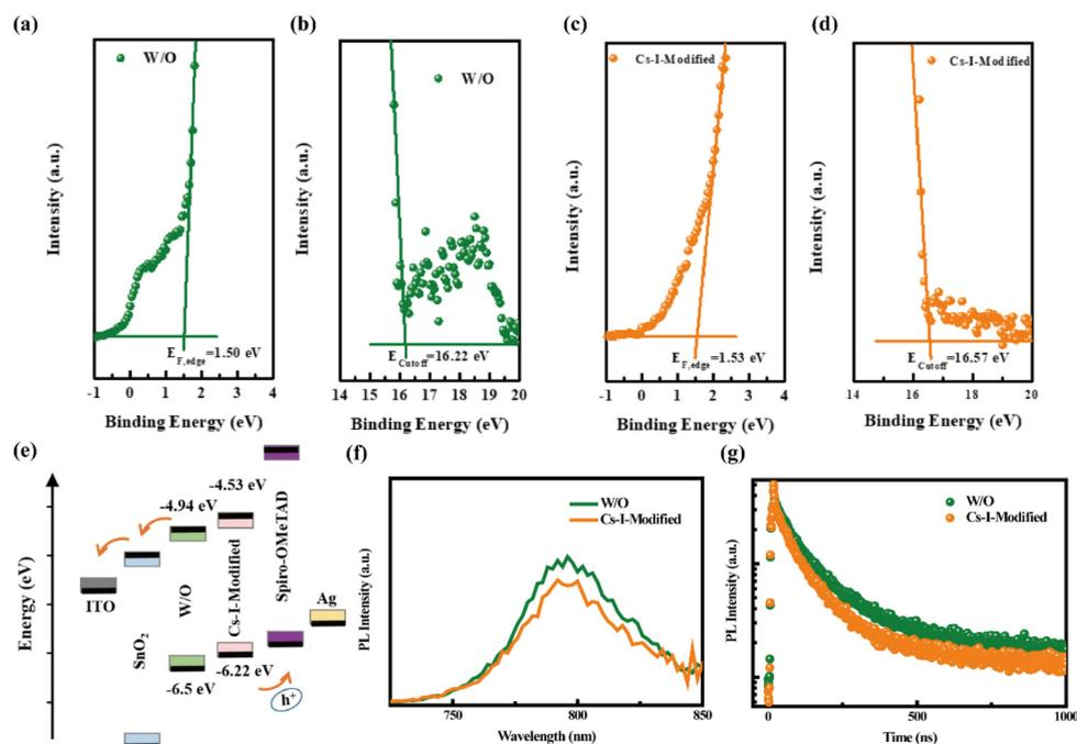
**Fig. 4** The UPS spectra showing the  $E_{Cutoff}$  and  $E_{F,edge}$  of (a), (b) the W/O film; (c) and (d) the Cs-I-modified film; (e) energy level diagram of device components. (f) PL spectra and (g) time-resolved PL spectra for the samples of Quartz/pristine PVSK/Spiro-OMeTAD and Quartz/Cs-I-modified PVSK/Spiro-OMeTAD.
