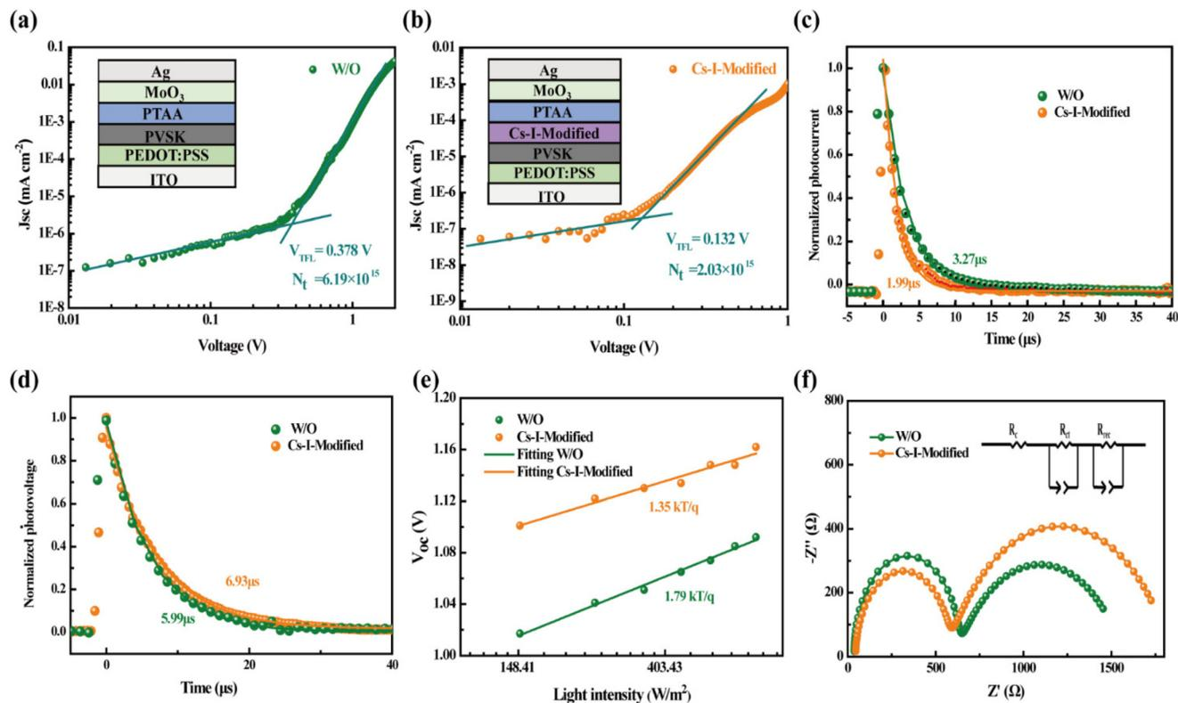
**Fig. 5** Dark  $J-V$  curves of the hole-only devices with the structures of (a) ITO/PEDOT:PSS/Perovskite/PTAA/MoO<sub>3</sub>/Ag and (b) ITO/PEDOT:PSS/Cs-I-modified Perovskite/PTAA/MoO<sub>3</sub>/Ag. (c) TPC and (d) TPV decay curves, (e)  $V_{oc}$  as a function of light intensities, and (f) Nyquist plots of the PSCs without and with Cs-I modification.
