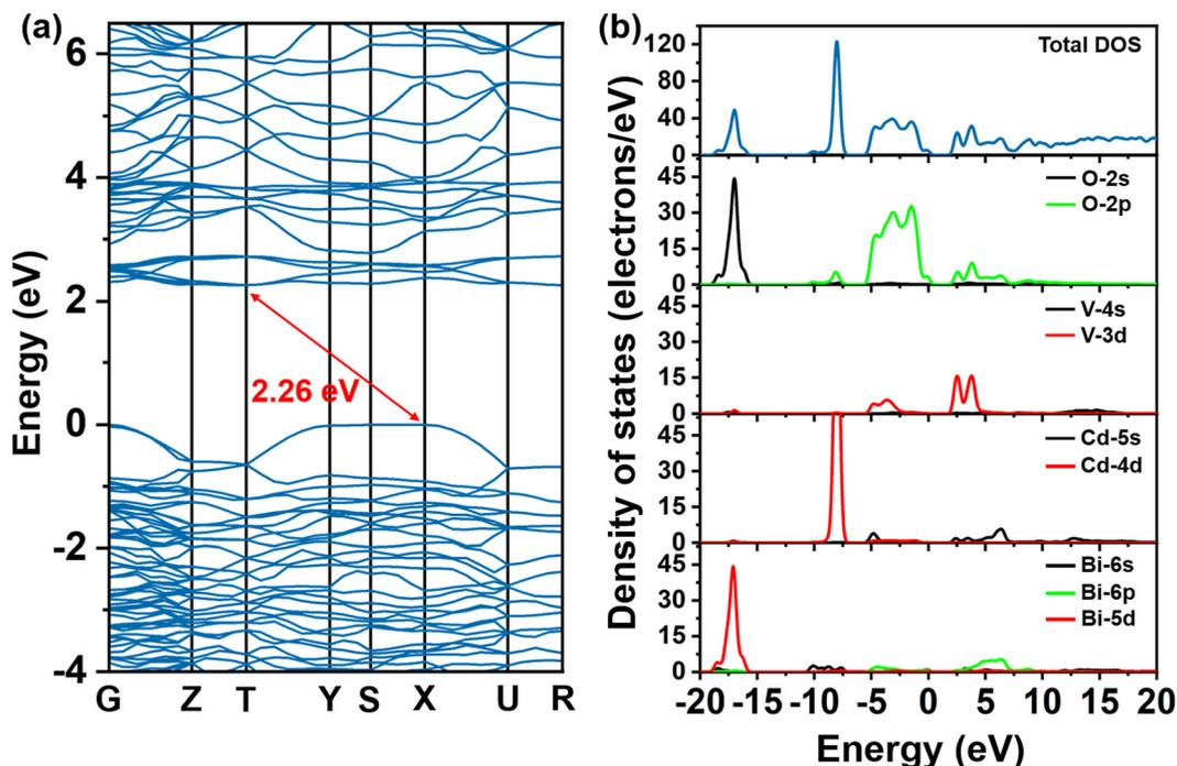
Fig. 4 (a) Band structure of CBVO. (b) Partial and total density of states of CBVO.
