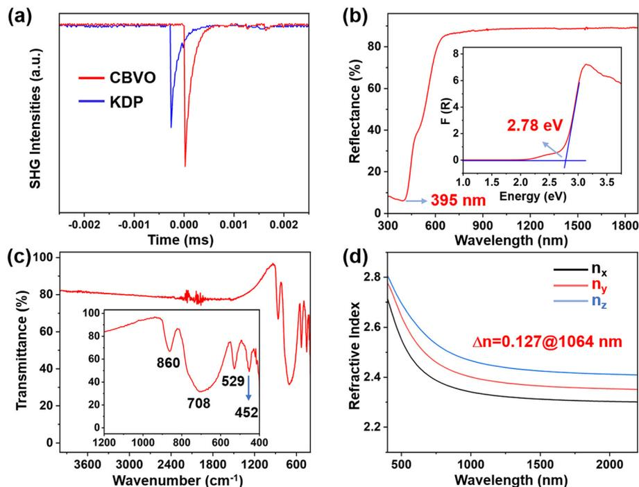
**Fig. 3** Optical characterization. (a) SHG intensity of the CBVO compound compared to that of the KDP reference. (b) UV-vis-NIR diffuse reflectance spectra and band gap of CBVO. (c) IR spectrum of CBVO. (d) Calculated refractive indices of CBVO.
