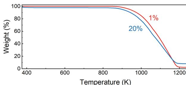
**Fig. 2** TGA curves for CsPbCl<sub>3</sub> powders composed of 1 and 20% of Nd<sup>3+</sup> ions.
