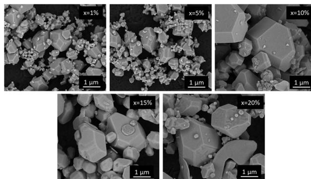
**Fig. 3** SEM images of the CsPbCl<sub>3</sub> perovskite powders containing different concentrations of Nd<sup>3+</sup> ions.
