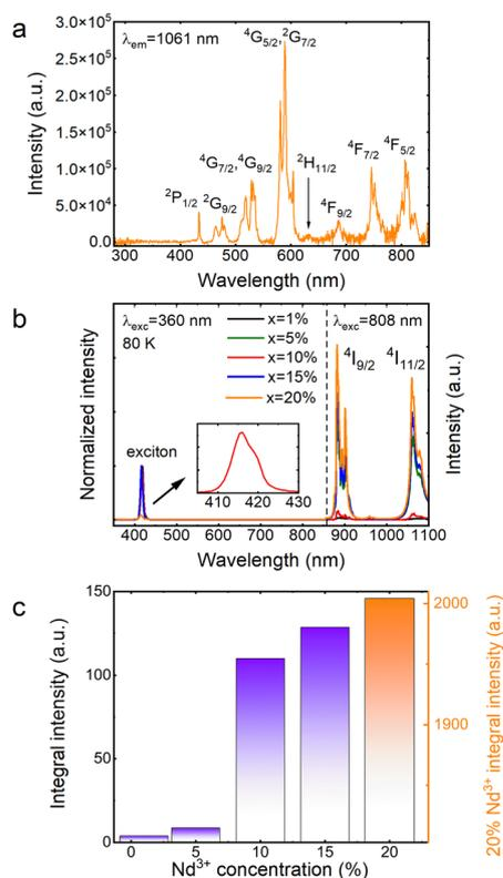
**Fig. 7** Excitation spectra of  $\text{CsPbCl}_3:20\%\text{Nd}^{3+}$  at 300 K (a). Emission spectra of the  $\text{CsPbCl}_3:x\%\text{Nd}^{3+}$  perovskite powders recorded at 80 K together with an inset showing an enlarged exciton spectrum of the  $\text{CsPbCl}_3:10\%\text{Nd}^{3+}$  sample (b), and integral intensities of  $\text{Nd}^{3+}$  emission (c). For clarity in (c), the sample containing 20% of the dopant is shown on a larger scale.
