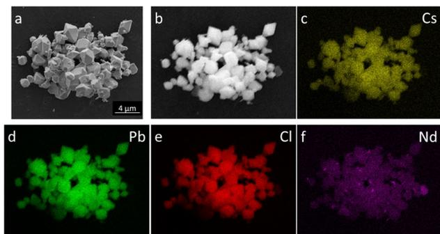
Fig. 4 SEM image (a) and EDS elemental mapping (b–f) of the CsPbCl<sub>3</sub>:10%Nd<sup>3+</sup> perovskite powder.
