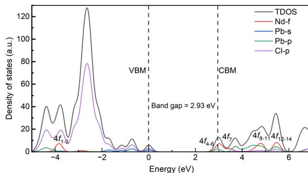
**Fig. 9** Density of state diagrams calculated for CsPbCl<sub>3</sub>:Nd<sup>3+</sup>. The labels VBM and CBM represent the maximum of the valence band and the minimum of the conduction band, respectively. The positions of the fourteen 4f dopant energy states are denoted by 4f<sub>n</sub> (n = 1–14).
