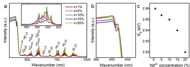
Fig. 6 Diffuse reflectance spectra of the CsPbCl<sub>3</sub>:*x*%Nd<sup>3+</sup> perovskite powders (a) together with an enlarged spectrum showing the exciton band (b) and energy gap values as a function of dopant concentration (c).
