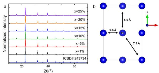
**Fig. 1** X-ray diffraction patterns of the CsPbCl<sub>3</sub>:x%Nd<sup>3+</sup> perovskite powders (a) and a simplified unit cell scheme of an undoped sample (b).
