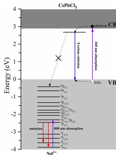
**Fig. 10** Electronic energy level scheme determined for the CsPbCl<sub>3</sub>:Nd<sup>3+</sup> perovskite powder.
