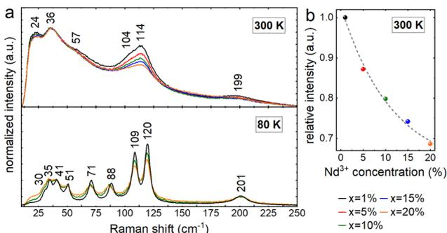
Fig. 5 Raman spectra of the CsPbCl<sub>3</sub> perovskite powders containing different concentrations of Nd<sup>3+</sup> ions at 300 and 80 K (a) together with the relative intensity change of the band at 114 cm<sup>-1</sup> at 300 K (b).
