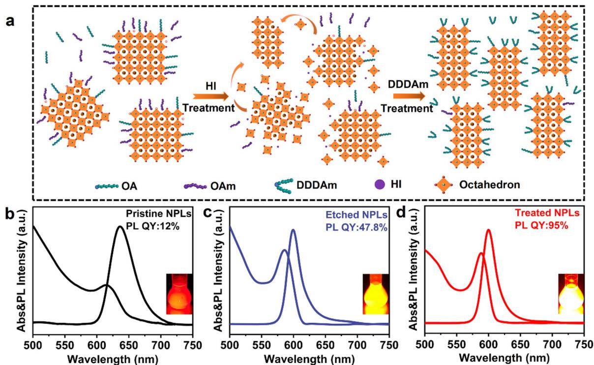
**Fig. 1** HI-assisted ligand treatment method for the synthesis of CsPbI<sub>3</sub> NPLs. (a) Schematic outlines the synthesis strategy. (b–d) Absorption and PL spectra of (b) pristine CsPbI<sub>3</sub> NPLs, (c) etched CsPbI<sub>3</sub> NPLs using HI, and (c) treated CsPbI<sub>3</sub> NPLs using HI and the DDDAm ligand. The insets display digital photos of colloidal solutions on these NPLs under 365 nm UV lamp excitation.
