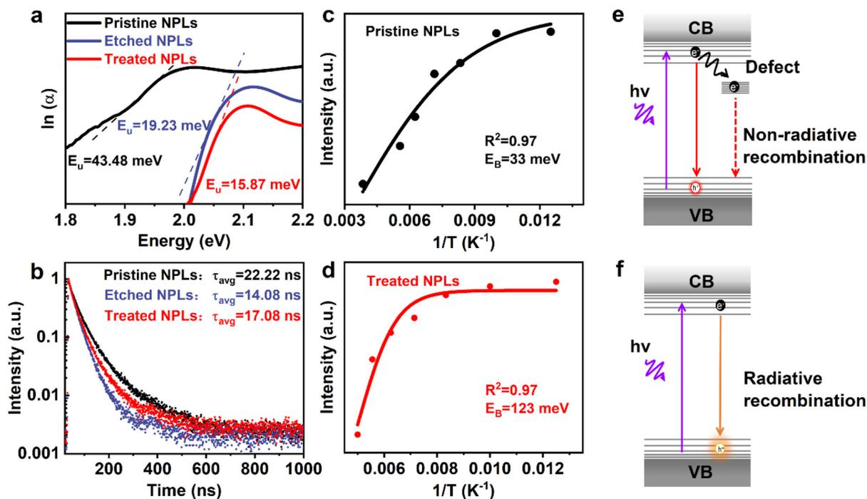
Fig. 4 The photophysical properties of CsPbI<sub>3</sub> NPLs. (a) Urbach energy spectra and (b) PL decay curves of the pristine, etched, and treated NPLs. (c and d) The function and fitting curve of the reciprocal of the PL intensity and temperature for both the pristine and treated NPLs. (e and f) Schematic representations of the PL radiative recombination process for the pristine and treated NPLs.
