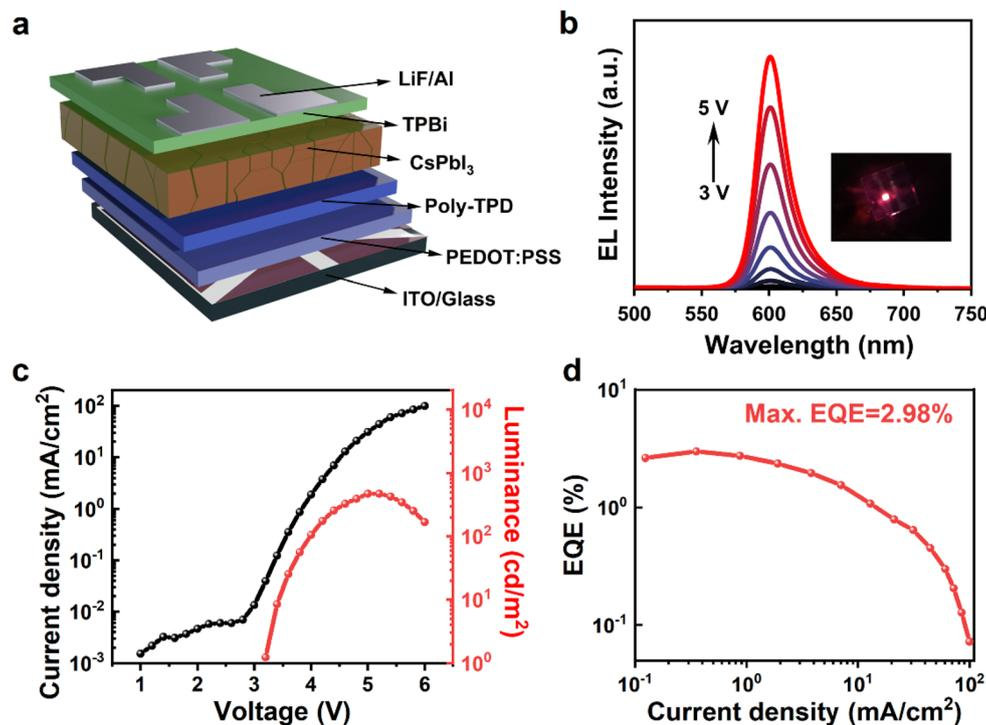
**Fig. 6** EL performance of PeLEDs based on the treated CsPbI<sub>3</sub> NPLs. (a) Structure and (b) EL spectra of PeLEDs under different voltage drivings. (c) Current density–brightness–voltage relationship, and (d) EQE–brightness relationship of PeLEDs.
