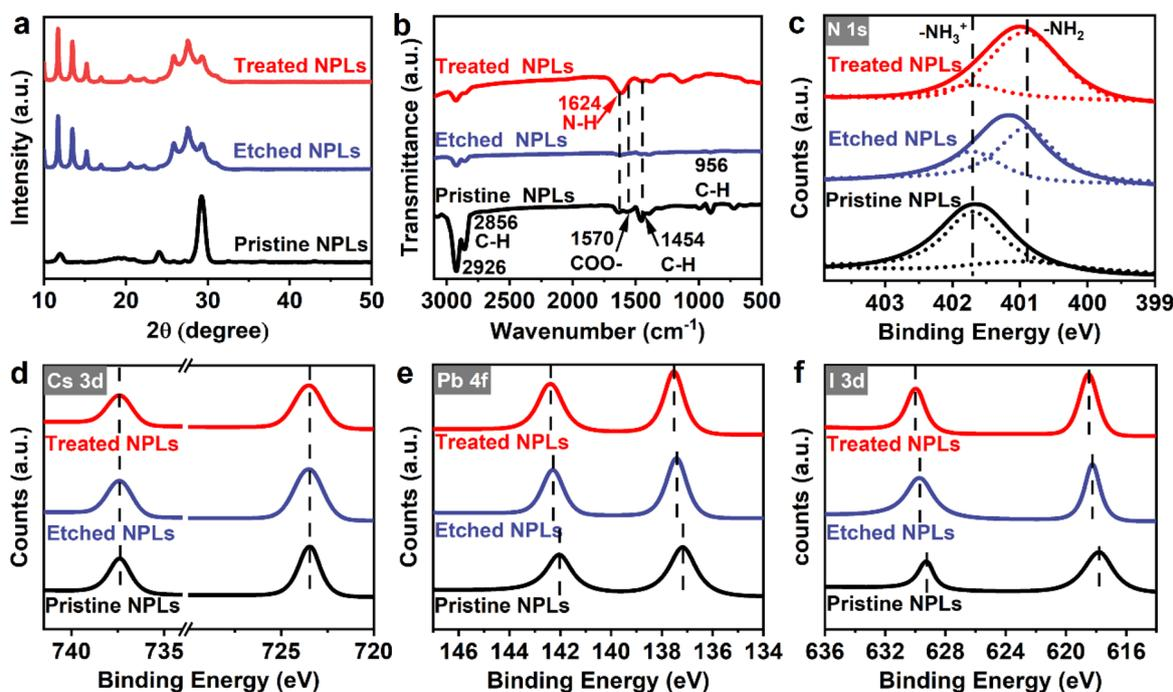
Fig. 3 The microstructure of the pristine, etched, and treated CsPbI<sub>3</sub> NPLs. (a) XRD patterns. (b) FTIR spectra. (c) N 1s, (d) Cs 3d, (e) Pb 4f, and (f) I 3d of XPS spectra.
