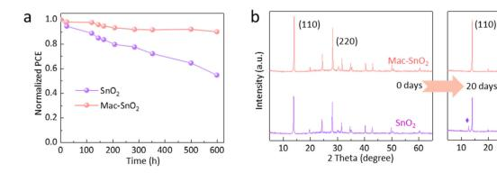
Fig. 7 (a) Normalized PCEs of SnO<sub>2</sub> and Mac-SnO<sub>2</sub> PSCs placed in the ambient environment (25–30 °C, 30%–40% humidity). (b) XRD spectra of the  $SnO_2$ /perovskite and Mac- $SnO_2$ /perovskite before and after exposure to an air environment with 30%-40% humidity for 20 days.
