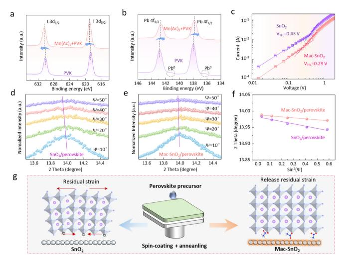
Fig. 4 XPS spectra of (a) Pb 4f and (b) I 3d for the perovskite and Mn(Ac)<sub>2</sub> + perovskite. (c) Dark I-V curves based on SnO<sub>2</sub> and Mac-SnO<sub>2</sub>. Depthdependent GIXRD patterns of the (d)  $SnO_2$ /perovskite and (e) Mac- $SnO_2$ /perovskite, and their (f) linear fits of  $2\theta - \sin^2 \Psi$ . (g) Residual stress diagram of the SnO<sub>2</sub>/perovskite and Mac-SnO<sub>2</sub>/perovskite.
