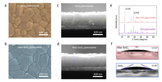
Fig. 3 Top-view and cross-section SEM images of perovskite layers grown on (a and c) SnO<sub>2</sub> and (b and d) Mac-SnO<sub>2</sub> ETL. (e) XRD patterns of the SnO<sub>2</sub>/perovskite and Mac-SnO<sub>2</sub>/perovskite. (f) The water contact angles on SnO<sub>2</sub> and Mac-SnO<sub>2</sub> films.
