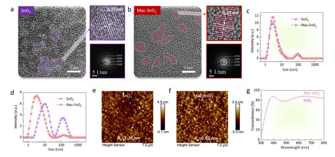
Fig. 1 HRTEM images and their SAED images of (a) SnO<sub>2</sub> and (b) Mac-SnO<sub>2</sub>. (c) Particle-size distribution of fresh SnO<sub>2</sub> and Mac-SnO<sub>2</sub> solutions. (d) Particle-size distribution of 72 h-aged SnO<sub>2</sub> and Mac-SnO<sub>2</sub> solutions. AFM topographical images of (e) SnO<sub>2</sub> and (f) Mac-SnO<sub>2</sub> films. (g) Optical transmittance spectra of ITO/SnO<sub>2</sub> and ITO/Mac-SnO<sub>2</sub> films.
