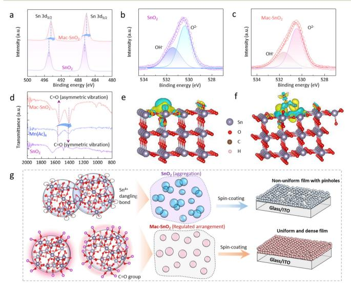
Fig. 2 XPS spectra of (a) Sn 3d and (b and c) O 1s for SnO<sub>2</sub> and Mac-SnO<sub>2</sub>. (d) FTIR spectra of SnO<sub>2</sub> and Mac-SnO<sub>2</sub>. Side view of (e) SnO<sub>2</sub>-O<sub>V</sub> and the charge density difference of (f) SnO<sub>2</sub>-O<sub>v</sub>/Ac<sup>-</sup>. (g) Schematic of the distribution of SnO<sub>2</sub> and Mac-SnO<sub>2</sub> QDs in the solutions and films.
