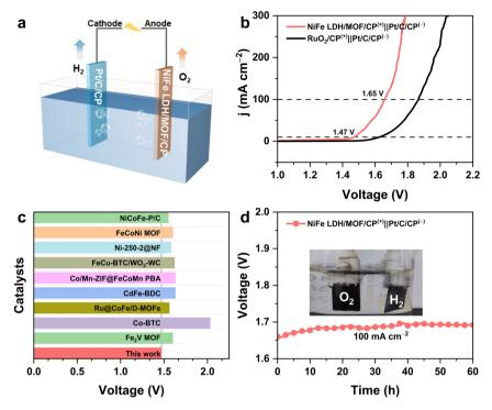
Fig. 5 (a) Schematic diagram of the overall water splitting (OWS) electrolyzer, (b) polarization curves of NiFe LDH/MOF/ $CP^{(-)}$  ||Pt/ $C/CP^{(-)}$  and RuO<sub>2</sub>/ $CP^{(+)}$ ||Pt/ $C/CP^{(-)}$ , (c) comparison of cell voltages with the recently reported catalysts at 10 mA cm<sup>-2</sup>, and (d) long-term stability test of NiFe LDH/MOF/ $CP^{(+)}$ ||Pt/ $C/CP^{(-)}$  at 100 mA cm<sup>-2</sup> in 1.0 M KOH.
