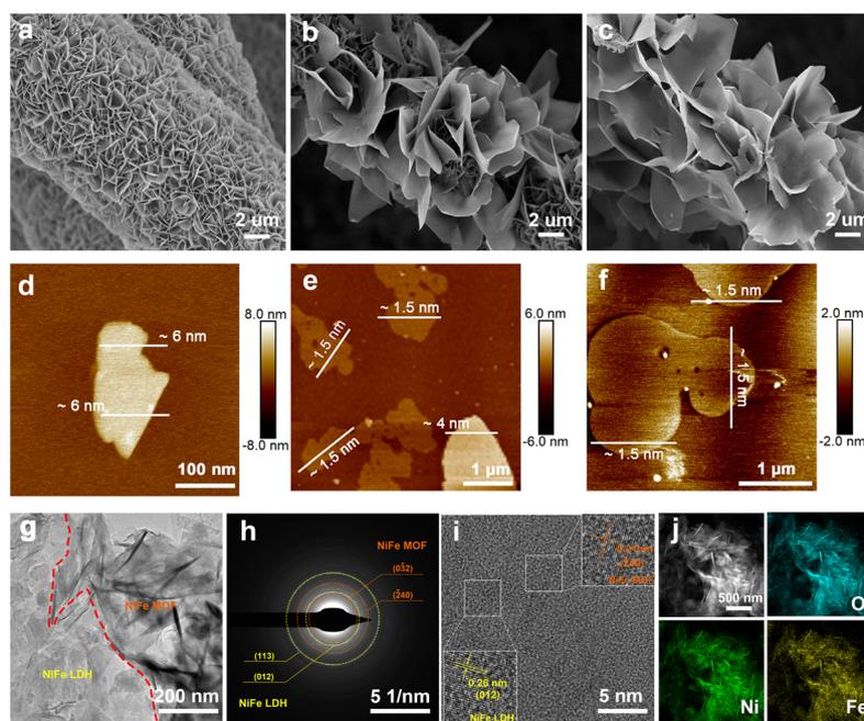
**Fig. 2** (a–c) SEM and (d–f) AFM images of the NiFe LDH (a and d), NiFe LDH/MOF (b and e) and NiFe MOF (c and f). (g) TEM image, (h) SAED pattern, (i) HR-TEM image, and (j) HAADF-STEM image and the corresponding elemental mappings of the NiFe LDH/MOF.
