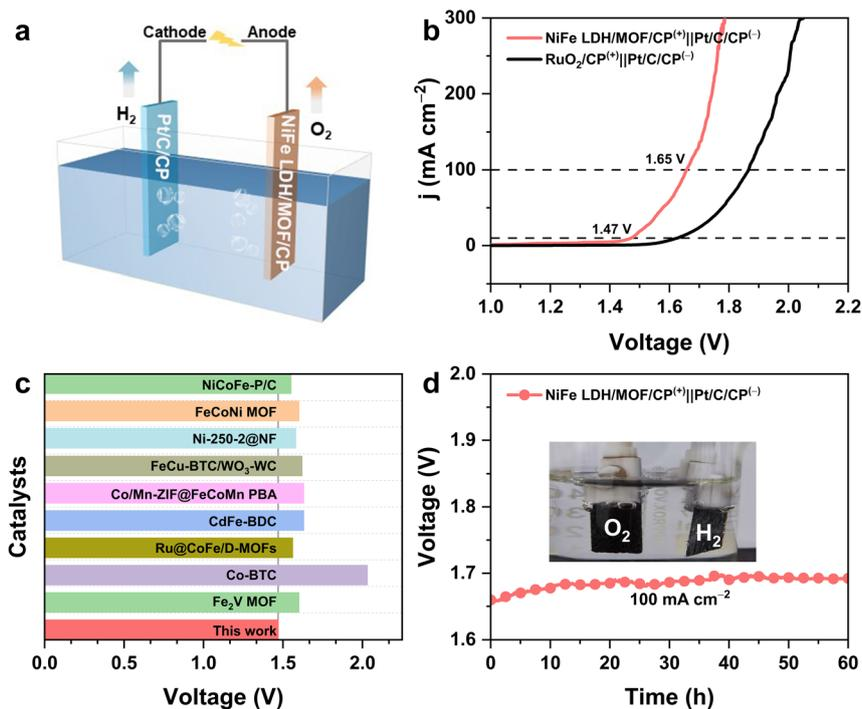
**Fig. 5** (a) Schematic diagram of the overall water splitting (OWS) electrolyzer, (b) polarization curves of NiFe LDH/MOF/CP<sup>(+)</sup>||Pt/C/CP<sup>(-)</sup> and RuO<sub>2</sub>/CP<sup>(+)</sup>||Pt/C/CP<sup>(-)</sup>, (c) comparison of cell voltages with the recently reported catalysts at 10 mA cm<sup>-2</sup>, and (d) long-term stability test of NiFe LDH/MOF/CP<sup>(+)</sup>||Pt/C/CP<sup>(-)</sup> at 100 mA cm<sup>-2</sup> in 1.0 M KOH.
