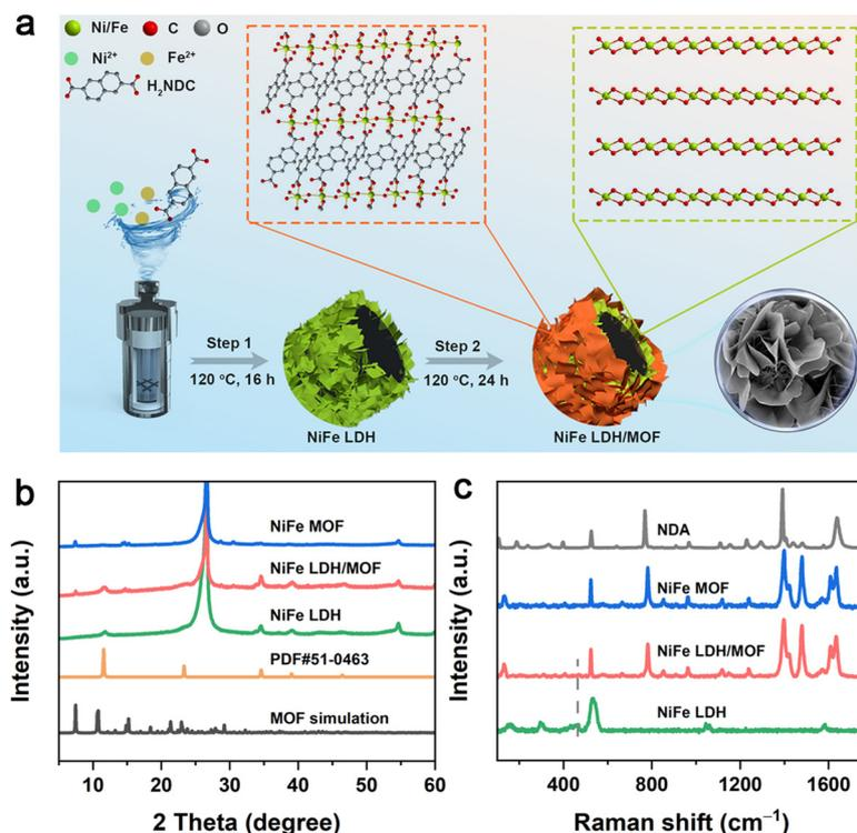
**Fig. 1** (a) Schematic illustration of the synthesis of the NiFe LDH/MOF. (b) XRD patterns and (c) Raman spectra of the NiFe LDH, NiFe LDH/MOF, and NiFe MOF, respectively.
