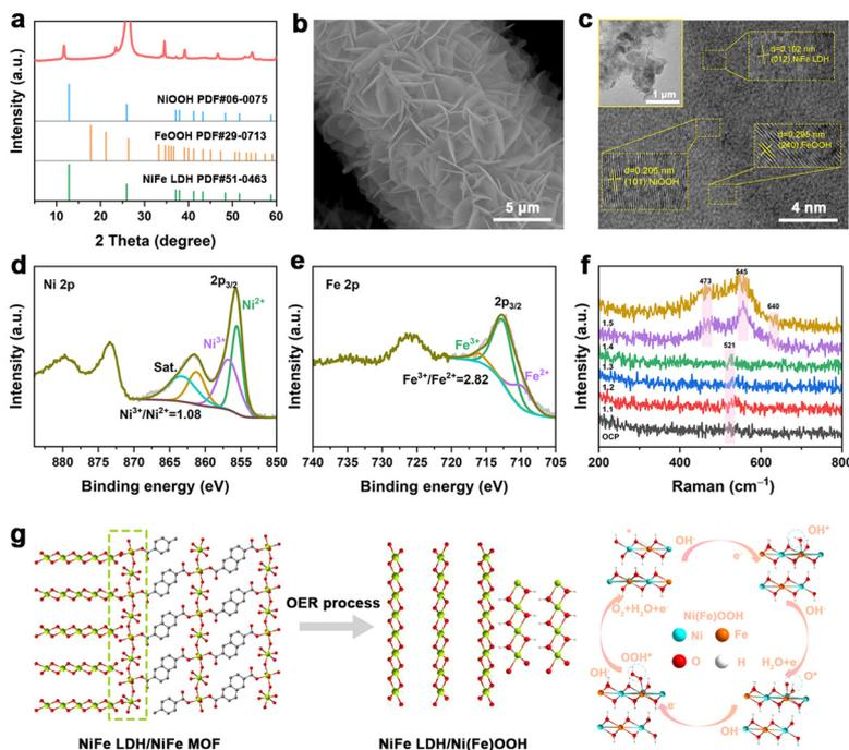
**Fig. 6** (a) XRD, (b) SEM image, (c) HR-TEM (inset TEM) image, high-resolution (d) Ni 2p and (e) Fe 2p XPS spectra of the NiFe LDH/MOF after OER stability, and (f) *in situ* Raman spectra of the NiFe LDH/MOF at different potentials (vs. RHE). (g) Proposed catalytic mechanism of the NiFe LDH/MOF in the OER process.
