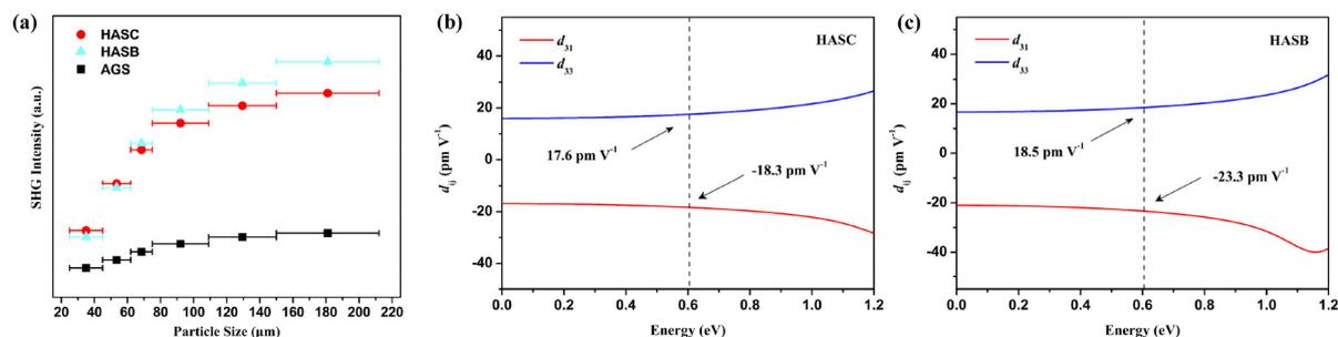
Fig. 3 (a) Particle size-dependent SHG intensity curves for HASC and HASB with reference of AGS under a 2050 nm laser. Calculated independent NLO coefficients for (b) HASC and (c) HASB.
