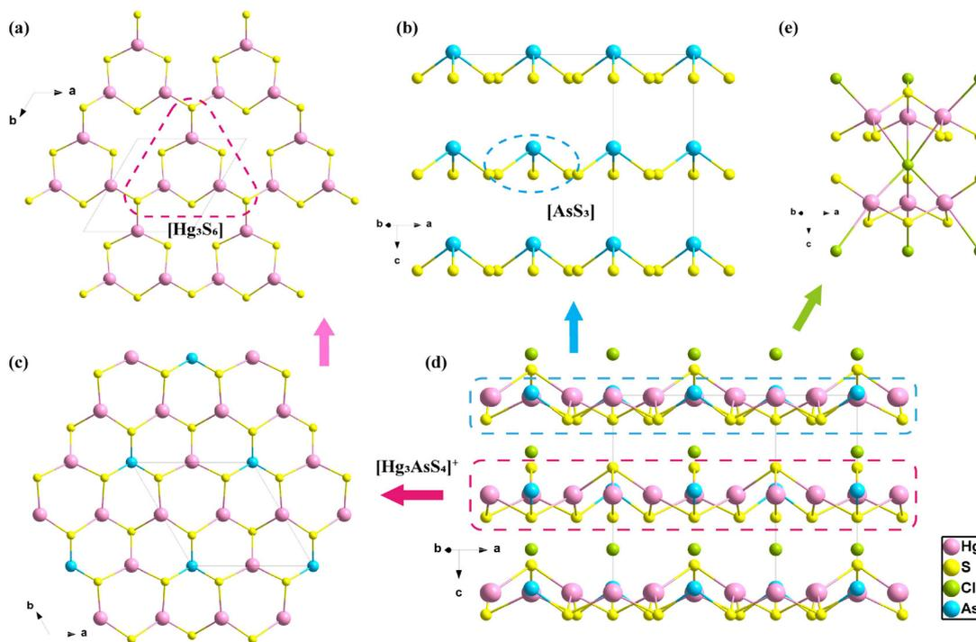
**Fig. 1** (a) [Hg<sub>3</sub>S<sub>6</sub>] unit and [Hg<sub>3</sub>S<sub>6</sub>] groups, (b) [AsS<sub>3</sub>] unit and [AsS<sub>3</sub>] array, (c) infinite [Hg<sub>3</sub>AsS<sub>4</sub>]<sup>+</sup> layer, (d) crystal structure of HASC viewed in the (010) plane, and (e) connection of Cl atoms.
