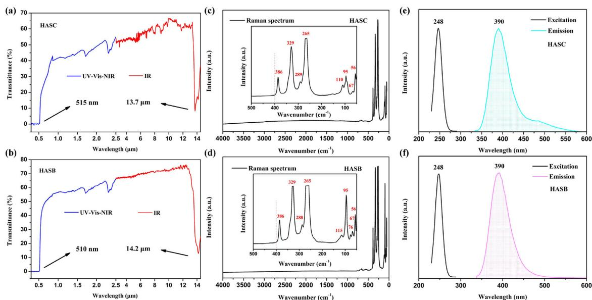
**Fig. 2** UV-Vis-NIR and IR transmittance spectra for (a) HASC and (b) HASB, Raman spectrum for (c) HASC and (d) HASB, and PL excitation and emission spectra for (e) HASC and (f) HASB, respectively.
