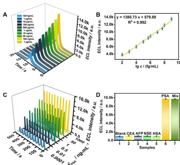
**Fig. 4** (A) ECL intensity–potential profiles of the constructed CRE aptasensor with various concentrations of the target PSA ( $100 \text{ fg mL}^{-1} \sim 1 \mu\text{g mL}^{-1}$ ). (B) Corresponding calibration plot of the constructed CRE aptasensor for PSA detection. (C) Stability of the constructed CRE aptasensor. (D) Selectivity of the constructed CRE aptasensor with relevant interfering molecules. Error bars = SD, ( $n = 3$ ).
