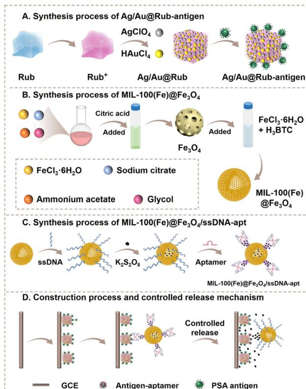
**Scheme 1** Synthesis process of (A) Ag/Au@Rub-antigen, (B) MIL-100(Fe)@Fe<sub>3</sub>O<sub>4</sub>, and (C) MIL-100(Fe)@Fe<sub>3</sub>O<sub>4</sub>/ssDNA-apt, and (D) the construction process and controlled release mechanism of the CRE aptasensor.
