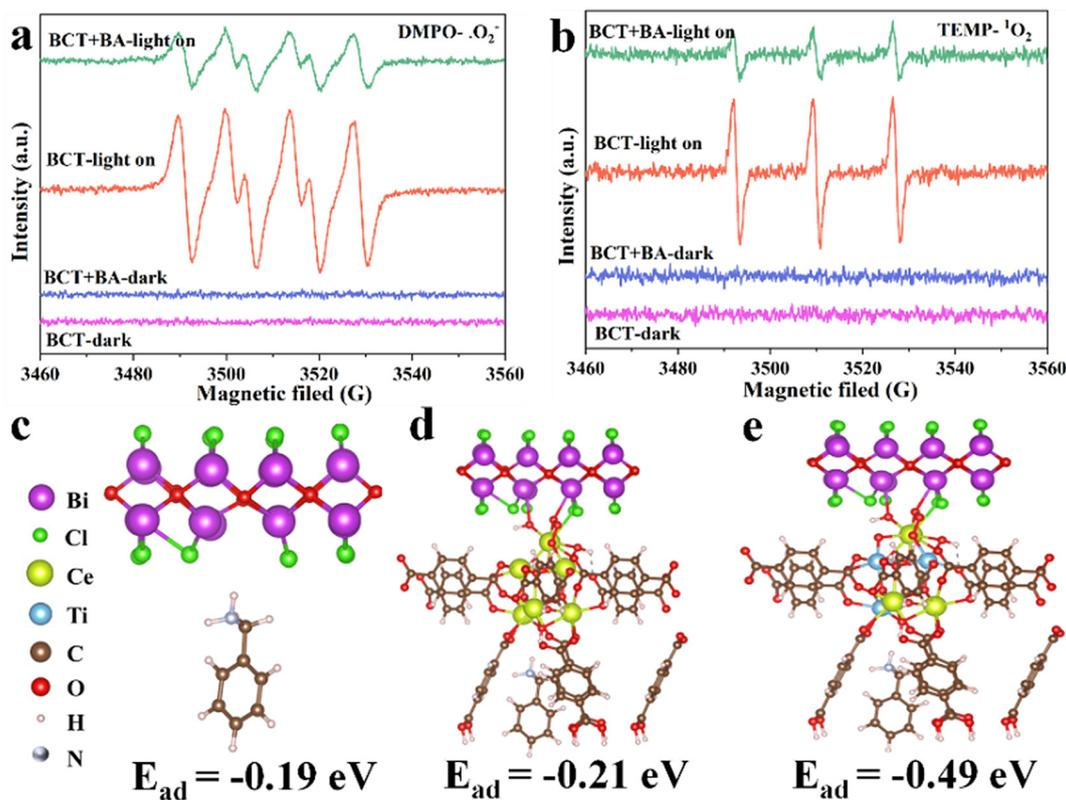
**Fig. 7** EPR spectra of the samples after mixing (a) TEMP and (b) DMPO solutions with BCT and  $O_2$  in the absence or presence of benzylamine under visible light irradiation or in the dark. Optimized adsorption structures: (c) BA on BiOCl, (d) the BiOCl/UIO-66(Ce) heterojunction, and (e) the BiOCl/UIO-66(Ce/Ti) heterojunction. Purple, green, yellow, blue, brown, red, pink, and blue grey atoms are Bi, Cl, Ce, Ti, C, O, H, and N respectively.
