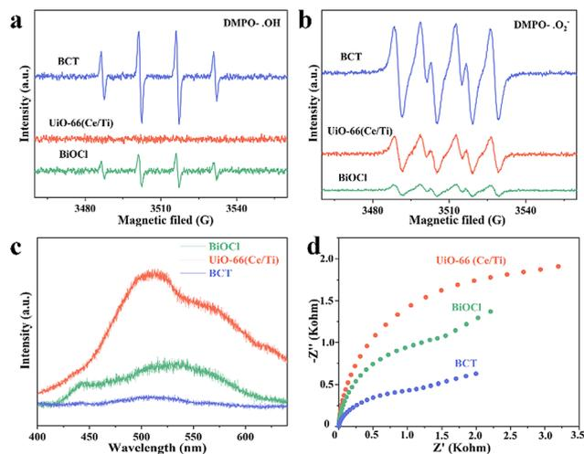
**Fig. 6** Electron paramagnetic resonance (EPR) spectra of (a) DMPO-<sup>•</sup>OH adducts and (b) DMPO-<sup>•</sup>O<sub>2</sub><sup>−</sup> adducts over BiOCl, UiO-66(Ce/Ti), and BCT under illumination for 2 min. (c) Steady-state photoluminescence (PL) spectra and (d) electrochemical impedance spectroscopy (EIS) spectra of BiOCl, UiO-66(Ce/Ti), and BCT.
