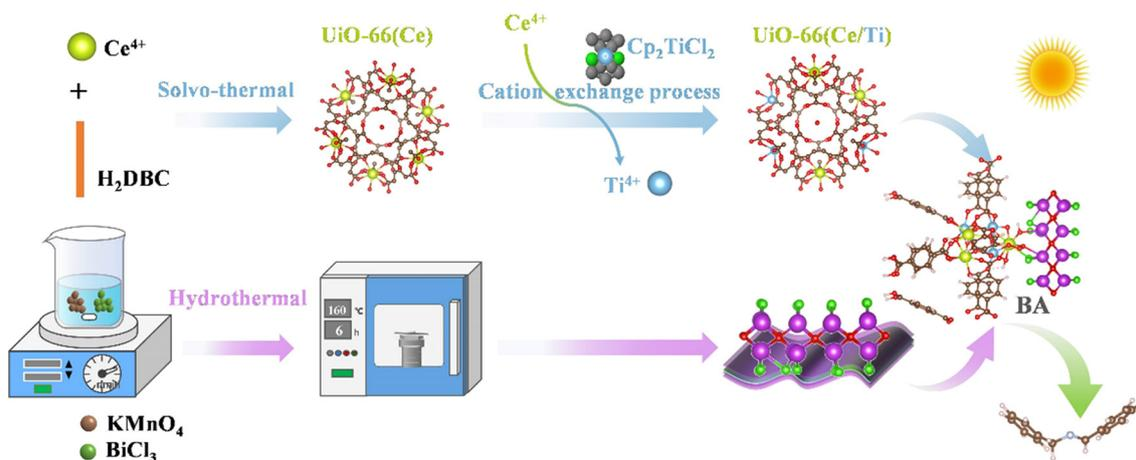
**Scheme 1** Synthetic illustration of the BCT heterojunction photocatalyst.
