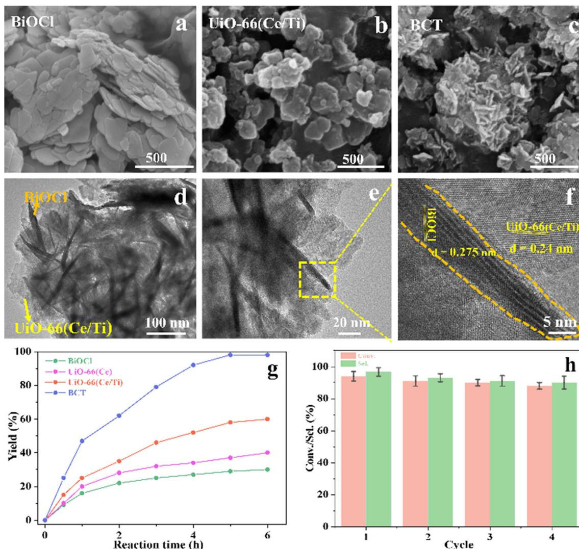
**Fig. 1** SEM images of the as-prepared samples: (a) BiOCl, (b) UiO-66(Ce/Ti) and (c) BCT. HRTEM images of BCT (d–f). (g) Time course of yields of different catalysts. (h) Photoactivity of recycled BCT. Reaction conditions: 0.2 mmol substrate, 20 mg of catalyst,  $\text{O}_2$  atmosphere, 3 mL of  $\text{H}_2\text{O}$ ,  $\lambda > 400$  nm. Yields were determined by GC-MS.
