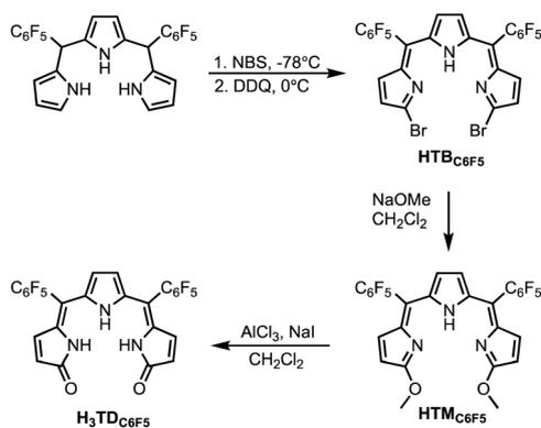
**Scheme 1** Synthesis of 5,10-di(pentafluorophenyl)-tripyrin-1,14-dione (H<sub>3</sub>TD<sub>C<sub>6</sub>F<sub>5</sub></sub>).
