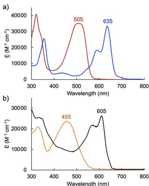
**Fig. 4** UV-visible absorption spectra of (a) tripyrrin  $HTM_{C_6F_5}$  (red) and its Pd(II) complex  $[Pd(TM_{C_6F_5}^{\#})]$  (blue) in  $CH_2Cl_2$  and (b) tripyrindione  $H_3TD_{C_6F_5}$  (orange) and complex  $[TBA][Pd(TD_{C_6F_5}^{3-})(H_2O)]$  (black) in  $CH_2Cl_2$ .
