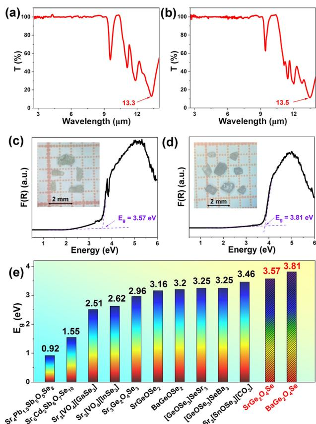
**Fig. 2** Optical property characterization of  $\text{AEGe}_2\text{O}_4\text{Se}$  (AE = Sr and Ba): (a and b) IR transmittance spectra; (c and d) UV-vis-NIR absorption spectra (inset: photographs of crystals); (e) comparison of the experimental  $E_g$  value of reported oxyselenides.
