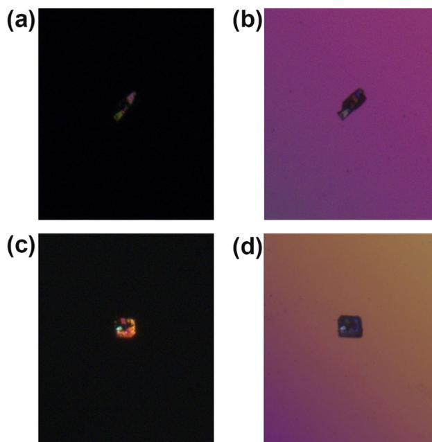
**Fig. 3** Changes in the interference color of (a and b)  $\text{SrGe}_2\text{O}_4\text{Se}$  and (c and d)  $\text{BaGe}_2\text{O}_4\text{Se}$  crystals before and after complete extinction.
