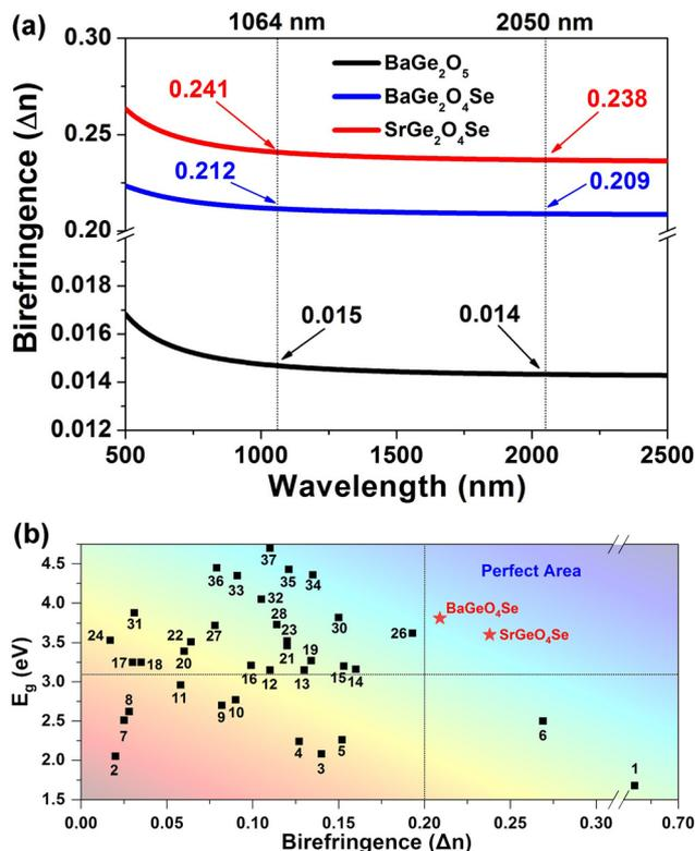
Fig. 5 (a) Calculated birefringence ( $\Delta n$ ) of oxide  $\text{BaGe}_2\text{O}_5$  and oxychalcogenide  $\text{AEGe}_2\text{O}_4\text{Se}$  (AE = Sr and Ba); (b) comparison of the experimental  $E_g$  and calculated  $\Delta n$  values of known oxychalcogenides (1–37) listed in Table S4.†
