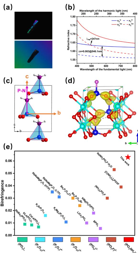
**Fig. 4** (a) Photograph of  $\text{NaPO}_3\text{NH}_3$  in the size of 19.64  $\mu\text{m}$ ; (b) calculated the refractive index of  $\text{NaPO}_3\text{NH}_3$ ; (c) the angular correlation between the P–N bond and the crystallographic axis  $c$  is  $0^\circ$ ; (d) the calculated electron density map of NPNH; (e) the birefringence of phosphates whose  $\lambda_{\text{cut-off}}$  below 200 nm.
