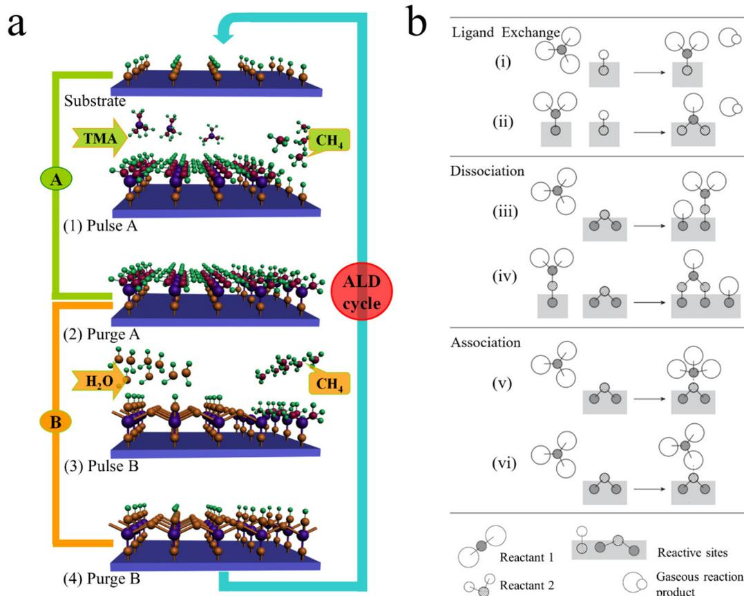
**Fig. 1** Schematic illustrations of (a) the ALD process, which is exemplified by that ALD Al<sub>2</sub>O<sub>3</sub> using TMA and water as precursors<sup>17</sup> and (b) the chemisorption mechanisms possible in ALD.<sup>22</sup> Reprinted with permission from ref. 17. Copyright (2012) John Wiley & Sons. Reprinted with permission from ref. 22. Copyright (2003) John Wiley & Sons.
