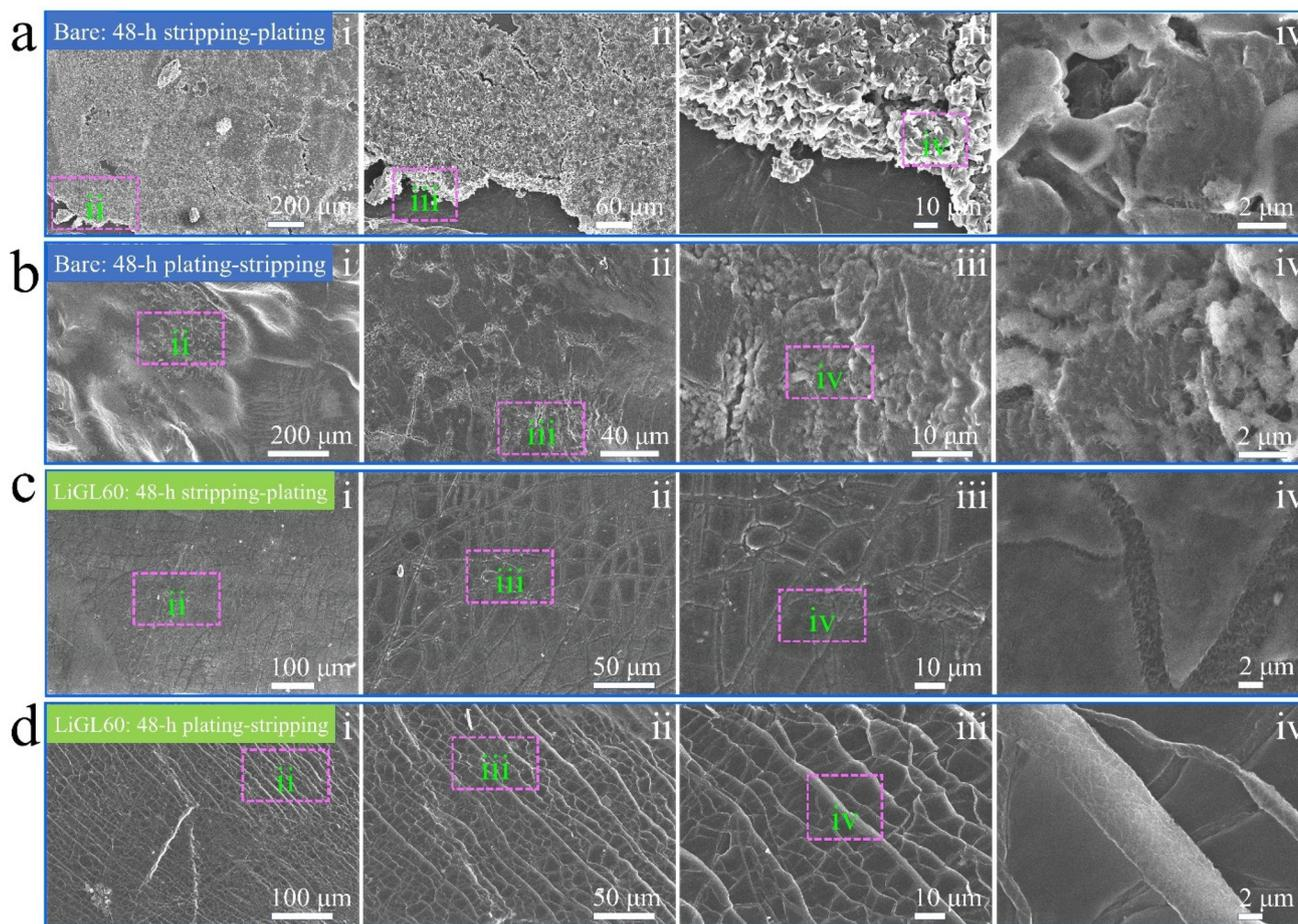
**Fig. 8** SEM observations of the morphological changes of Li electrodes:<sup>137</sup> (a and b) bare Li electrode and (c and d) LiGL60 electrode after one 48 h stripping-plating at  $2 \text{ mA cm}^{-2}$ . LiGL60 indicates the LiGL coating of 60 MLD cycles. The electrolyte is 1 M LiTFSI in 1/1 volume ratio of DOL/DME. Reprinted (adapted) with permission from ref. 137 under a Creative Commons Attribution (CC BY) license.
