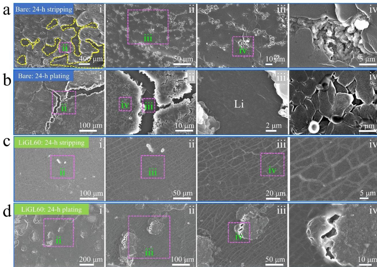
**Fig. 7** SEM observations of the morphological changes of Li electrodes:<sup>137</sup> (a and b) bare Li electrode and (c and d) LiGL60 electrode after one 24 h stripping (or plating) at 2 mA cm<sup>-2</sup>. LiGL60 indicates the LiGL coating of 60 MLD cycles. The electrolyte is 1 M LiTFSI in 1/1 volume ratio of DOL/DME. Reprinted (adapted) with permission from ref. 137 under a Creative Commons Attribution (CC BY) license.
