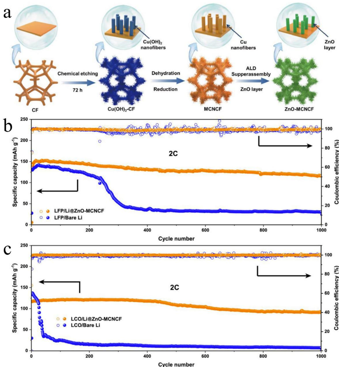
**Fig. 12** Effects of ALD ZnO on 3D hierarchical Cu foams.<sup>163</sup> (a) schematic illustration of the preparation process of Zn-MCNCF from CF. Electrochemical performance of (b) Li||LFP and (c) Li||LCO cells due to the adoption of Li@ZnO-MCNCF. The electrolyte is 1 M LiPF<sub>6</sub> in 1/1/1 volume ratio of EC/DMC/DEC. Reprinted (adapted) with permission from ref. 163. Copyright (2021) Elsevier.
