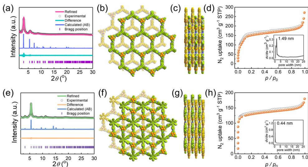
**Fig. 2** PXRD structural analyses of **JNM-18** (a) and **JNM-19** (e). Top and side views of the refined AB models of **JNM-18** (b and c) and **JNM-19** (f and g). Nitrogen adsorption (filled) and desorption (open) isotherm profiles of **JNM-18** (d) and **JNM-19** (h) at 77 K (the insets show pore size distribution profiles of **JNM-18** and **JNM-19** exhibiting a uniform pore size of 1.49 and 0.44 nm, respectively).
