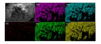
Fig. 2 EDS mapping of sodium (purple), zinc (blue), nitrogen (red), oxygen (green) and sulfur (yellow) on the 1 crystal (top left). The scale bar is 100  $\mu$ m.
