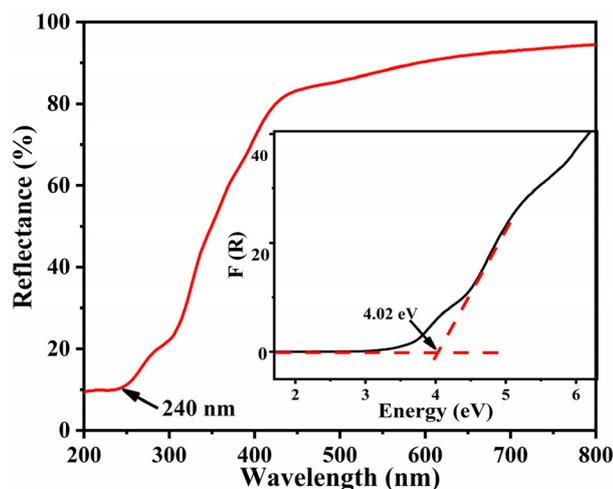
Fig. 4 UV-vis-NIR diffuse reflectance spectrum of **1**.
