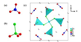
Fig. 3 (a)  $\pi$ -Conjugated [NO<sub>3</sub>] group. (b) Non- $\pi$ -conjugated heteroanion  $[SO_3S]$  group; (c) the crystal structure of 1 viewed along the c axis.
