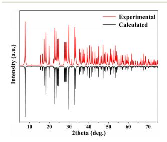
Fig. 1 Experimental and calculated XRD patterns of 1.
