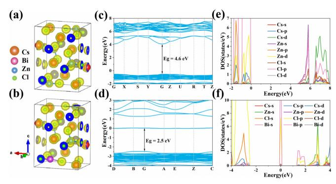
Fig. 5 (a and b) Calculated static charge-density, (c and d) calculated electronic band structure and (e and f) calculated PDOS of pristine Cs<sub>2</sub>ZnCl<sub>4</sub> and Cs<sub>2</sub>ZnCl<sub>4</sub>:Bi<sup>3+</sup> NCs, respectively.
