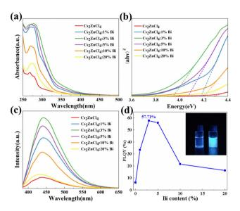
Fig. 2 (a) UV-Vis absorption spectra, (b) Tauc plots, (c) PL spectra, and (d) PLQY plots of Cs<sub>2</sub>ZnCl<sub>4</sub> NCs doped with different contents of Bi<sup>3+</sup>. The inset in (d) shows photographs of Cs<sub>2</sub>ZnCl<sub>4</sub> NCs and Cs<sub>2</sub>ZnCl<sub>4</sub>:3% Bi NCs under 365 nm UV.
