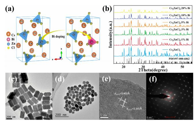
Fig. 1 (a) Crystal structures diagram of Cs<sub>2</sub>ZnCl<sub>4</sub> and Bi-doped Cs<sub>2</sub>ZnCl<sub>4</sub> NCs. (b) Comparison of PXRD patterns of Cs<sub>2</sub>ZnCl<sub>4</sub> NCs doped with different contents of Bi3+. TEM images of (c) Cs2ZnCl4 and (d) Cs2ZnCl4:3%Bi NCs. (e) HRTEM images of Cs2ZnCl4:3%Bi NCs. (f) SAED pattern of Cs<sub>2</sub>ZnCl<sub>4</sub>:3%Bi NCs.
