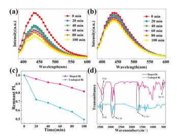
Fig. 7 (a and b) Antiwater stability and (c) Remnant PL spectra of pristine and Bi-doped Cs<sub>2</sub>ZnCl<sub>4</sub> NCs immersed in deionized water for different durations. (d) FTIR spectra of Bi-doped and pristine Cs<sub>2</sub>ZnCl<sub>4</sub> NCs before and after immersion.
