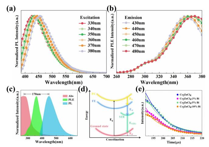
Fig. 3 (a) PLE spectra and (b) PL spectra for Cs<sub>2</sub>ZnCl<sub>4</sub>:3%Bi NCs. (c) Typical normalized absorption, excitation, and emission spectra of the as-synthesized Cs<sub>2</sub>ZnCl<sub>4</sub>:3%Bi NCs. (d) schematic diagram of self-trapping exciton emission. (e) Time-resolved PL spectrum of Cs<sub>2</sub>ZnCl<sub>4</sub> NCs doped with different contents of Bi3+ (excited at 365 nm, monitored at 445 nm).
