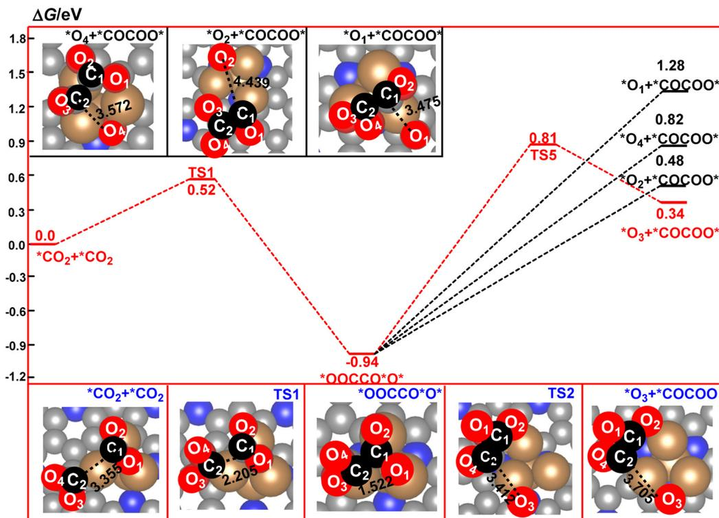
Fig. 5 Calculated reaction pathways for the formation and decomposition of the CO<sub>2</sub> dimer on the surface of the Cu<sub>4</sub>/N<sub>3</sub>GN catalyst.
