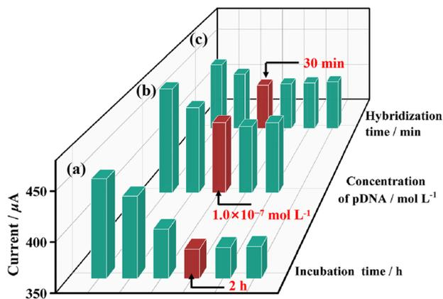
**Fig. 6** (a and b) DPV signal variation of Au/1-PEDOT/GCE with different pDNA incubation time and different pDNA concentration. (c) DPV signal variation of dhDNA/Au/1-PEDOT/GCE with different hybridization time. [DPV curves were measured in Fe-PBS (pH = 7.4)].
