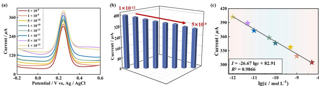
**Fig. 7** (a and b) DPV curves and signal intensity of pDNA/Au/1-PEDOT/GCEs capturing tDNA with different concentrations. (c) The linear relationship between the DPV signal intensity and  $\lg c(\text{tDNA})$ . All signals were measured in solution Fe-PBS (pH = 7.4).
