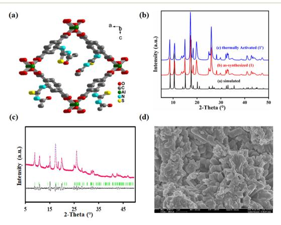
Fig. 1 (a) Simulated structure of 1. (b) PXRD profiles of 1 and 1' compared with simulated one. (c) Pawley refinement plot for the slow scan PXRD profile of 1' ( $R_{\rm wp}$  and  $R_{\rm p}$  are 5.4% and 3.8%, respectively). (d) FE-SEM image 1'.
