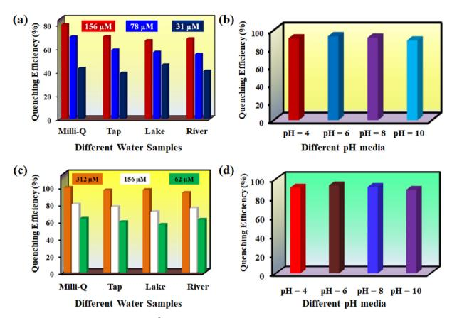
Fig. 6 Fluorescence quenching efficiency of (a) Hg<sup>2+</sup> and (c) ranitidine in different real water specimens and sensing ability of 1' in different pH media for (b) Hg<sup>2+</sup> and (d) ranitidine.
