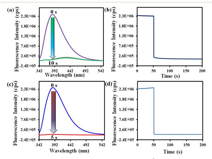
Fig. 3 Time-dependent variation in the fluorescence spectra of 1' after addition of (a) 100 μL of 10 mM Hq<sup>2+</sup> and (c) 200 μL of 5 mM ranitidine solution in aqueous and HEPES buffer media, respectively. Results of fluorescence kinetic experiments for (b) Hg<sup>2+</sup> and (d) ranitidine.
