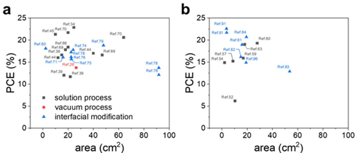
Fig. 8 The efficiency of (a) n-i-p and (b) p-i-n structured metal oxide-based PSMs over 1 cm<sup>2</sup> of the active or aperture area reported recently.
