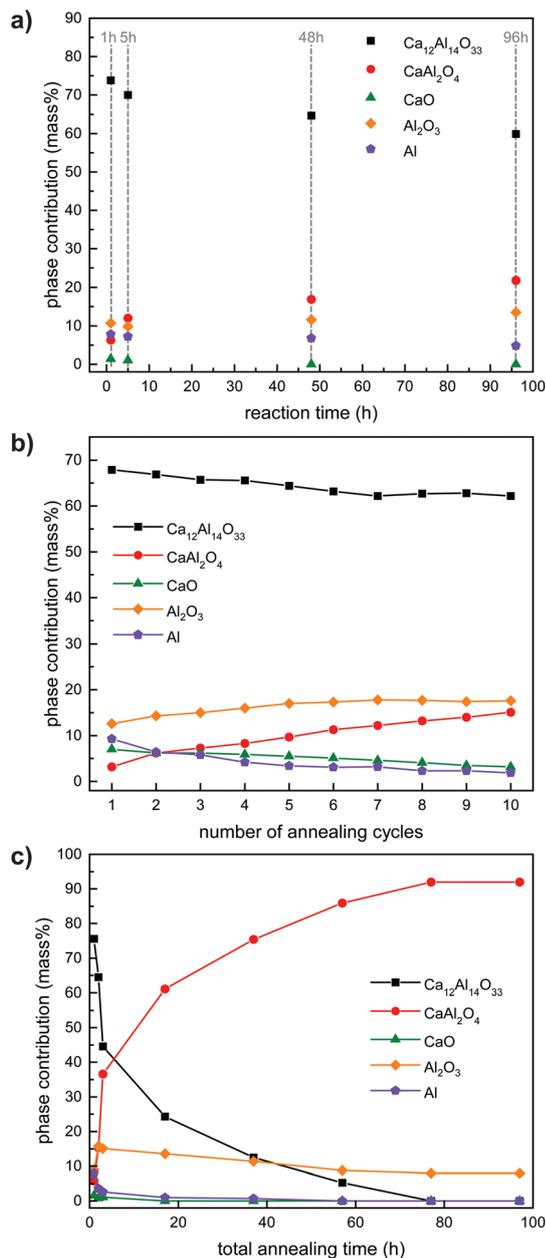
**Fig. 5** Results of the Rietveld refinements of the different oxidation approaches of CaAl<sub>2</sub>. (a) single long-term annealing, (b) repeated heating to 1273 K followed by grinding, and (c) increasing annealing times with intermediate grinding. The values are documented in Table 2.
