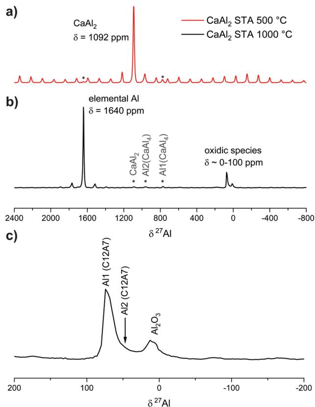
**Fig. 4**  $^{27}\text{Al}$  NMR investigations of the oxidation product (b) of  $\text{CaAl}_2$  (a). The full spectrum is shown in the top panels, a zoom of the region of the oxidic species at the bottom (c).
