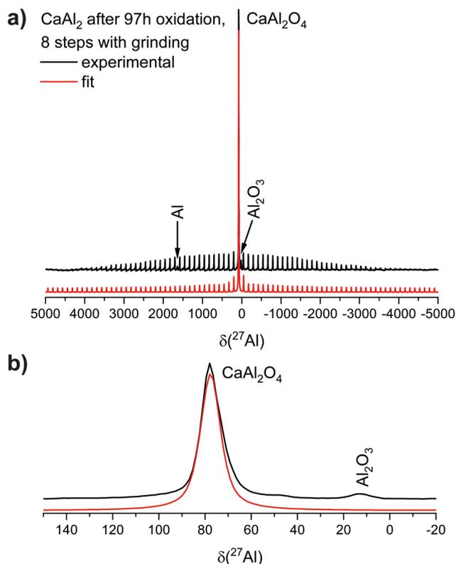
**Fig. 6**  $^{27}\text{Al}$  NMR investigations of the oxidation product of  $\text{CaAl}_2$  (black line) plotted versus the fitted data (red line). The full spectrum (a) is shown in the top panel, a zoom of the region (b) of the oxidic species at the bottom.
