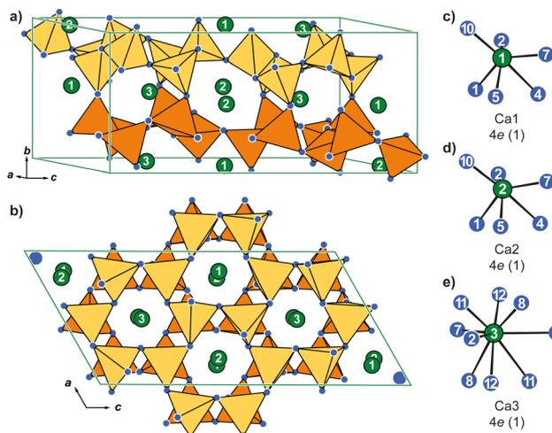
**Fig. 2** Unit cell of the of monoclinic  $\text{CaAl}_2\text{O}_4$  ( $P2_1/c$ , own type) in (a) side view and (b) along  $[010]$ . (c–e) Coordination environments of the Ca atoms. Wyckoff positions and site symmetries are given. Ca atoms are depicted in green, Al atoms as orange and O atoms as blue circles. The two layer-like arrangements of the  $[\text{AlO}_4]$  tetrahedra are depicted in light and dark orange.
