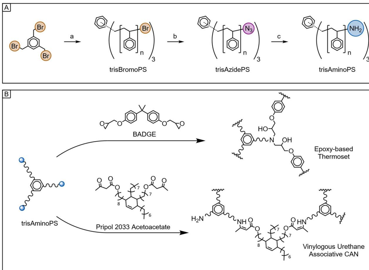
**Fig. 1** Overview of the reactions explored. (A) Synthetic pathway yielding trifunctional primary amine-terminated polystyrene: (a) ARGET ATRP of styrene initiated by 1,3,5-tris(bromomethyl)benzene, (b) nucleophilic substitution with sodium azide, (c) Staudinger reduction with tributylphosphine and water. (B) Crosslinking process using bisphenol A diglycidyl ether (BADGE) or Pripol 2033 acetoacetate to form a traditional epoxy-based network or a vinyllogous urethane CAN, respectively.
