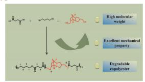
Synthesis of degradable polyester with high molecular weight and excellent mechanical properties through copolymerization modification of poly(butylene succinate)
