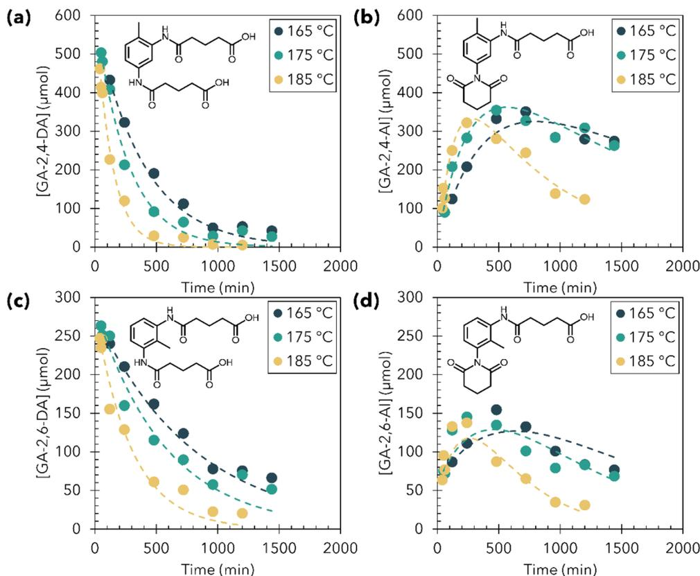
**Fig. 4** Concentrations (dots) and kinetic model fits (dashed lines) during M-PUF acidolysis with GA at 165–185 °C for (a) GA-2,4-DA, (b) GA-2,4-AI, (c) GA-2,6-DA, and (d) GA-2,6-AI. Data points were obtained via integration of peaks in <sup>1</sup>H NMR. Reaction conditions: 0.5 g M-PUF, 1.5 g GA under N<sub>2</sub> atmosphere.
