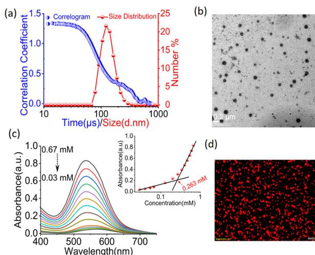
**Fig. 1** (a) DLS profile of the self-assembled amphiphile (nanoaggregate). (b) TEM image of the nanoaggregate. (c) Nile-red absorption spectra by varying the concentration of LPA. Inset shows a plot of absorption intensity vs. concentration for CAC calculation (CAC = 263  $\mu$ M). (d) Fluorescence microscopy image of a Nile red-encapsulated nanoaggregate.
