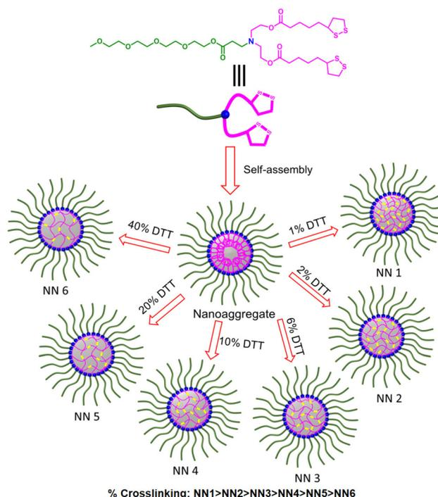
**Scheme 1** Chemical structure of the lipoic acid-based amphiphile. Self-assembly in aqueous medium and fabrication of a crosslinked poly(disulfide)s nanonetwork by varying the mol % of dithiothreitol (DTT) (schematic).
