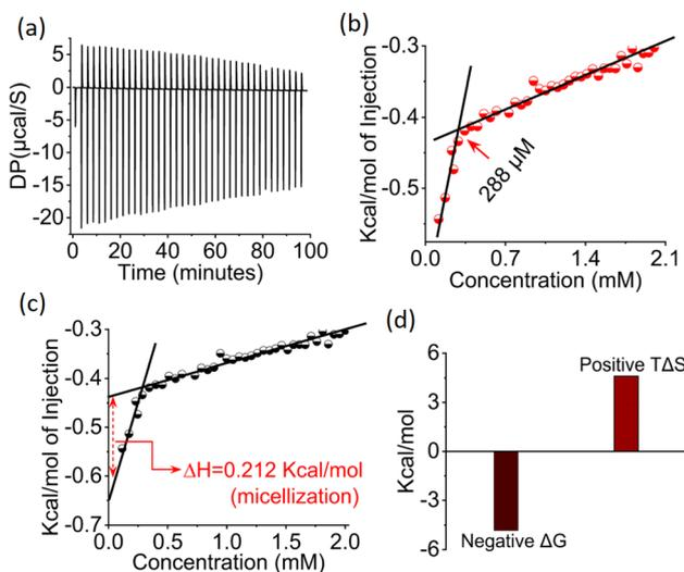
**Fig. 2** (a) Measurement of heat release by ITC upon injection of a nanoaggregate solution of LPA into pure water at 298 K. (b) CAC determination from a plot of enthalpy vs. concentration. (c) Calculation of  $\Delta H$  of aggregation from a plot of  $\Delta H$  vs. concentration. (d) Plot showing negative  $\Delta G$  and positive  $\Delta S$ . Experimental temperature = 298 K.
