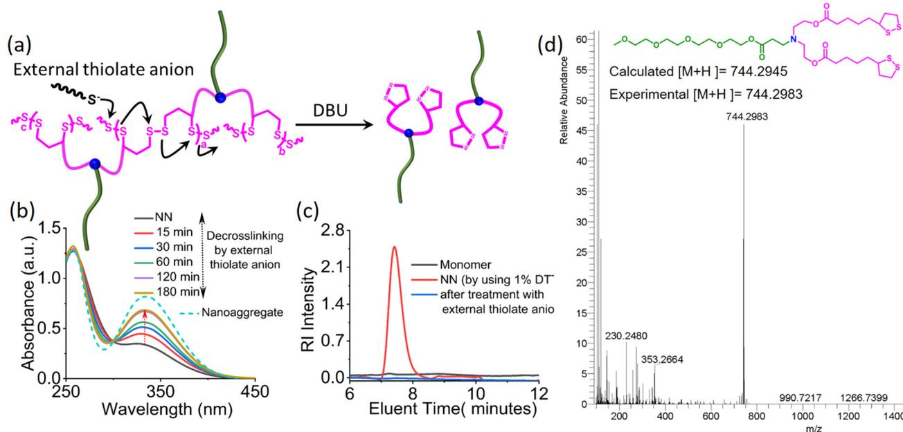
**Fig. 6** (a) Depolymerization by an external thiol in the presence of a DBU base (schematic). (b) Monitoring depolymerization by UV/visible spectroscopy, which shows increasing band intensity corresponding to the monomer at 335 nm. (c) GPC profile of poly(disulfide)s and depolymerized solution. (d) LC-MS profile of the depolymerized solution. Solvent for the column for GPC = DMF; measurement temperature = 30 °C.
