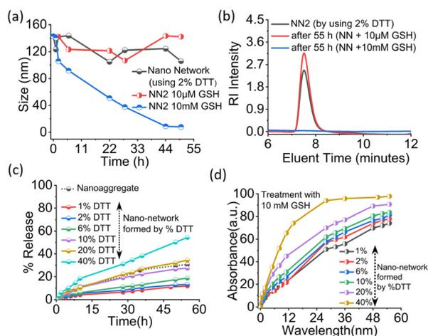
**Fig. 9** (a) Stability and degradation of nanonetworks under different GSH concentrations measured by DLS. (b) GPC profile of nanonetworks after and before treatment with various concentrations of GSH. Percent release of guest for all the nanonetwork and nanoaggregates in the (c) absence of GSH and (d) presence of GSH.
