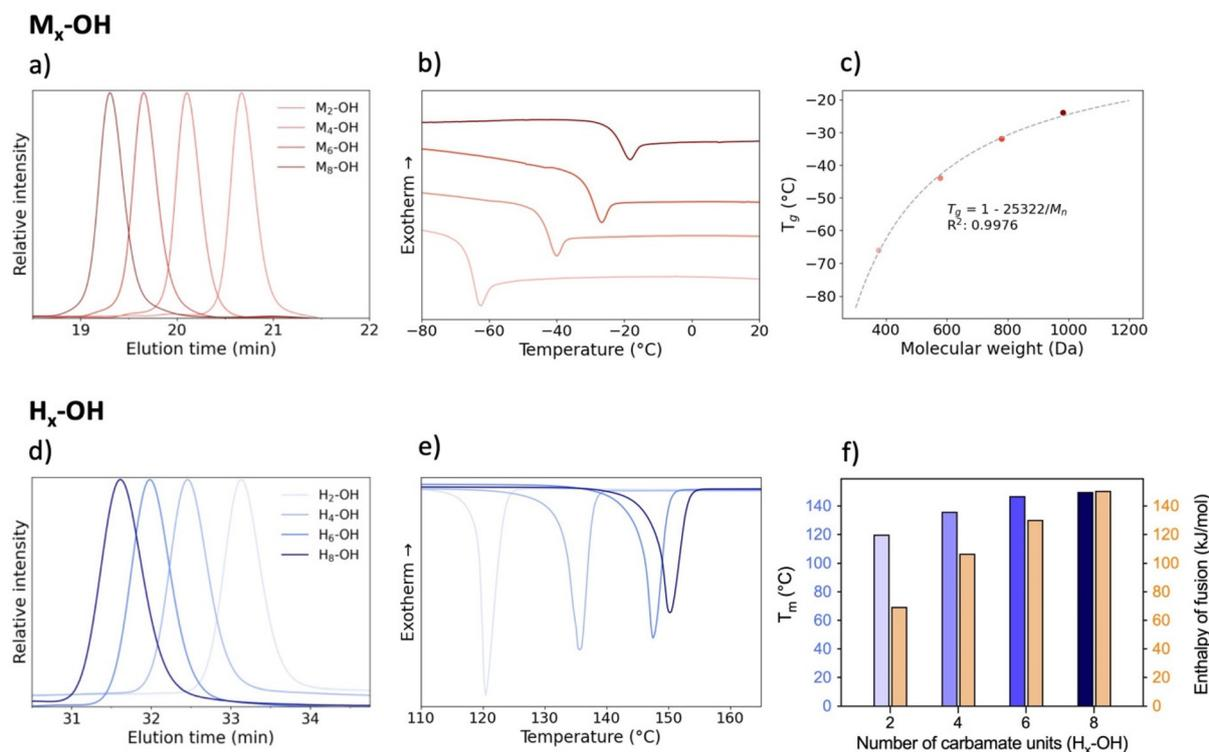
**Fig. 2** Characterization of the  $M_x$ -OH (top) and  $H_x$ -OH (bottom) oligomers. (a and d) SEC traces of the various macromolecules. (b and e) DSC curves showing the evolution of  $T_g$  or the melting temperature when varying the chain length for oligomers  $M_x$ -OH or  $H_x$ -OH, respectively. (c) Flory-Fox fitting showing the relationship between the  $T_g$  and the molecular weight. (f) Bar plots of the melting temperatures and enthalpy of fusion.
