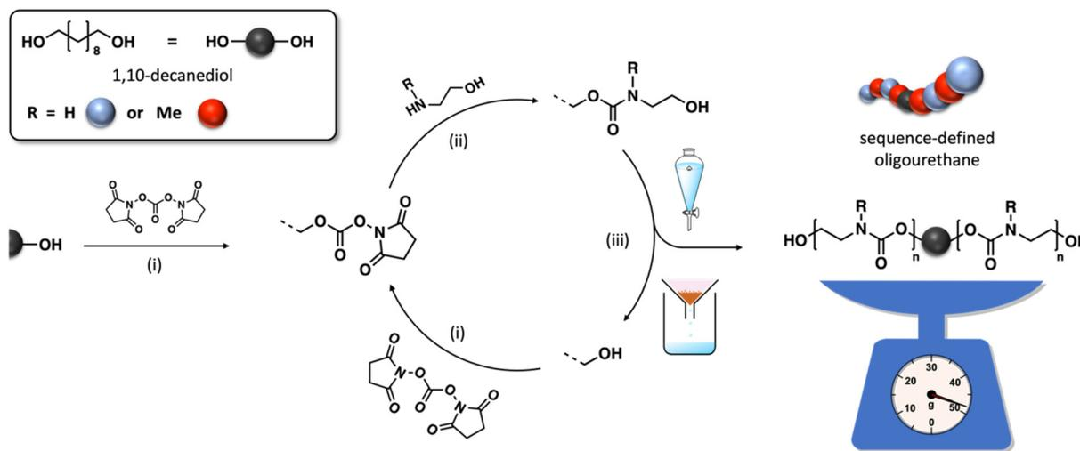
**Fig. 1** General synthesis protocol for the synthesis of uniform oligourethanes consisting of (i) an activation of the terminal alcohol groups to a carbamate, (ii) the subsequent chemoselective coupling with an aminoethanol and (iii) the purification with either an extraction or a precipitation.
