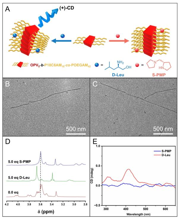
Fig. 5 (A) Schematic illustration of the co-assembly of  $OPV_5$ -b- $P18C6AM_{18}$ -co- $POEGAM_{42}$  with S-PMP and D-Leu. TEM images of the fiber-like micelles of  $OPV_5$ -b- $P18C6AM_{18}$ -co- $POEGAM_{42}$  formed with (B) S-PMP and (C) D-Leu, respectively. (D)  $^1H$  NMR spectra of  $P18C6AM_{18}$ -co- $POEGAM_{42}$  without and with the addition of S-PMP and D-Leu. (E) CD spectra of micellar solutions of  $OPV_5$ -b- $P18C6AM_{18}$ -co- $POEGAM_{42}$  formed with S-PMP and D-Leu.
