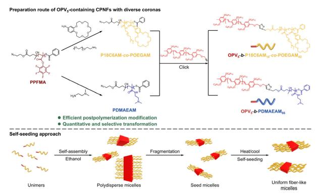
Scheme 1 Preparation route of OPV<sub>5</sub>-containing CPNFs with controlled length and varying coronas by the combination of pentafluorophenyl ester chemistry and the self-seeding approach of living CDSA.
