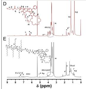
Fig. 1 (A) <sup>19</sup>F NMR spectra of azide-terminated PPFMA. <sup>19</sup>F NMR spectra of amidation reaction solutions of PPFMA-co-P18C6AM (B) and P18C6AMco-POEGAM (C). <sup>1</sup>H NMR spectra of azide-terminated P18C6AM-co-POEGAM (D) and OPV<sub>5</sub>-b-P18C6AM-co-POEGAM (E) (CD<sub>2</sub>Cl<sub>2</sub>).
