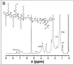
Fig. 6 (A)  $^{19}$ F NMR spectra of azide-terminated PPFMA and the reaction solution for the preparation of PDMAEAM<sub>66</sub>. (B)  $^{1}$ H NMR spectrum of OPV<sub>5</sub>-b-PDMAEAM<sub>66</sub> (CD<sub>2</sub>Cl<sub>2</sub>).
