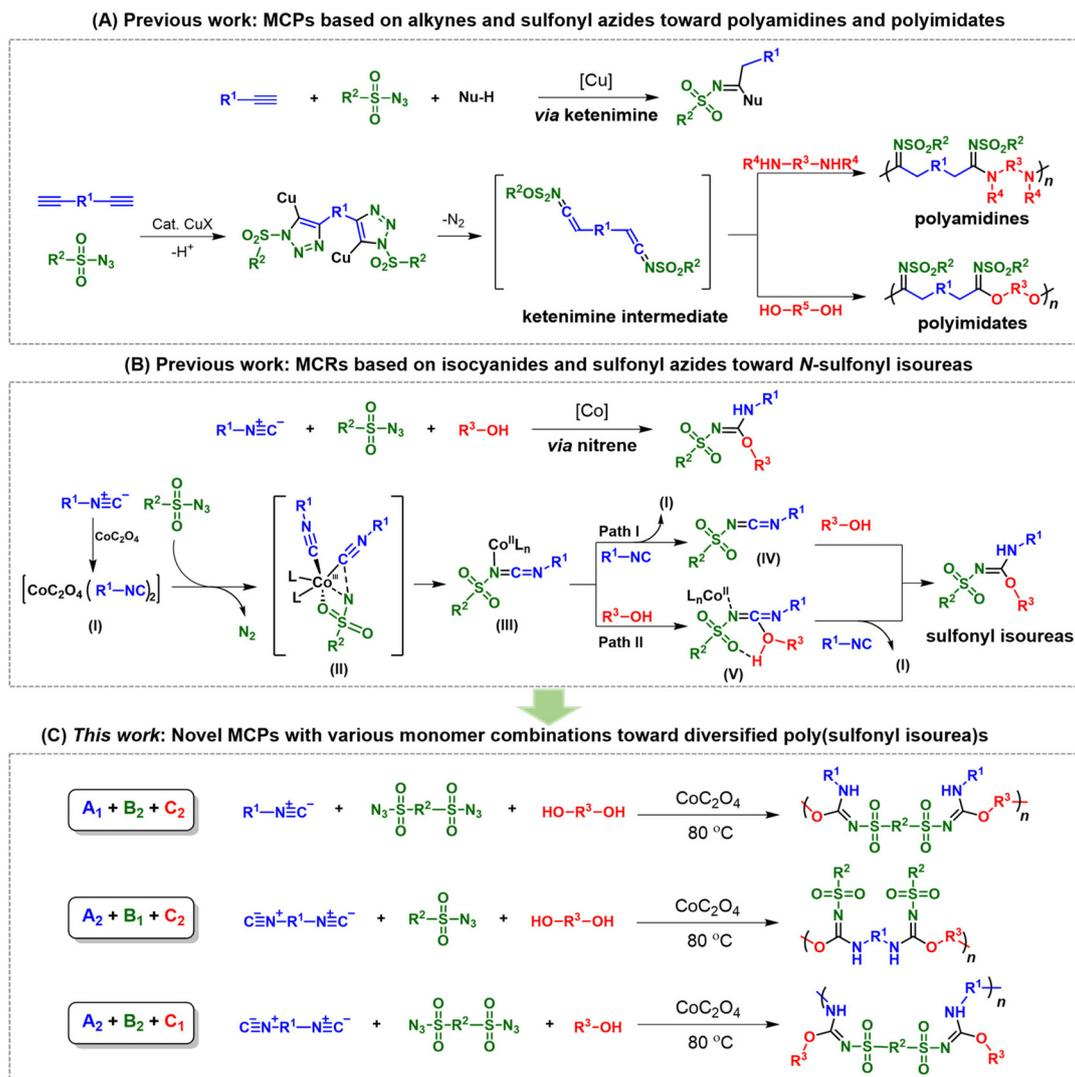
**Scheme 1** (A) Multicomponent polymerizations (MCPs) based on alkynes and sulfonyl azides; (B) multicomponent reactions (MCRs) based on isocyanides and sulfonyl azides toward *N*-sulfonyl isoureas; (C) MCPs reported in this work with various monomer combinations.
