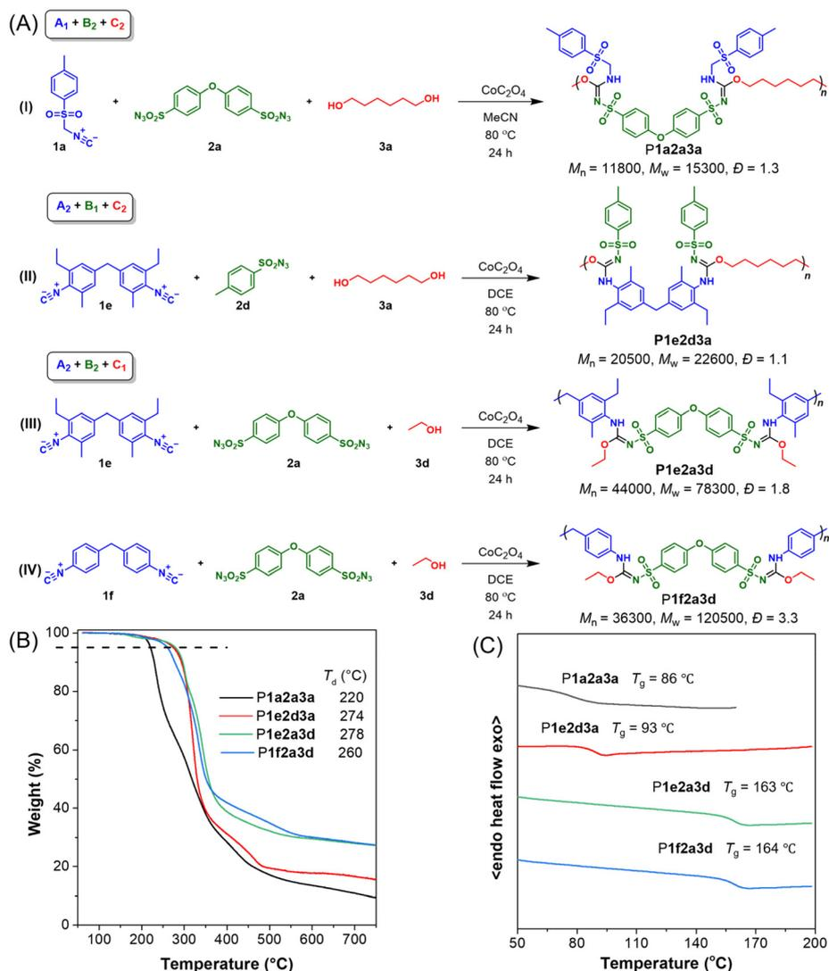
**Fig. 4** (A) The specific structures and molecular weights of **P1a2a3a**, **P1e2d3a**, **P1f2a3d** and **P1e2a3d**. (B) TGA thermograms of polymers recorded under nitrogen at a heating rate of  $10\text{ °C min}^{-1}$ . (C) DSC thermograms of polymers recorded under nitrogen during the second heating cycle at a heating rate of  $10\text{ °C min}^{-1}$ .
