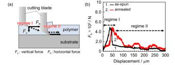
Fig. 4 (a) Schematic representation of SAICAS measurement, showing cutting modes and detecting forces along the directions vertical and horizontal to the interface. (b) Horizontal force ( $F_{\rm h}$ ) profile for the PMMA L & S film before and after annealing, measured in the direction perpendicular to the line pattern.
