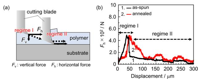
**Fig. 4** (a) Schematic representation of SAICAS measurement, showing cutting modes and detecting forces along the directions vertical and horizontal to the interface. (b) Horizontal force ( $F_h$ ) profile for the PMMA L&S film before and after annealing, measured in the direction perpendicular to the line pattern.
