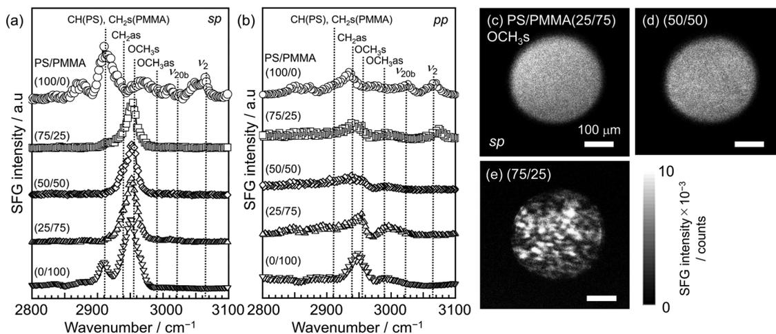
**Fig. 5** SFG spectra for PS/PMMA blend films with different bulk compositions with (a) sp and (b) pp polarization combinations. SFG images for PS/PMMA (c) (25/75), (d) (50/50), and (e) (75/25), respectively. All blend films were annealed at 433 K for 48 h under vacuum.
