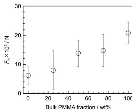
**Fig. 6** Bulk PMMA composition dependence of  $F_h$  for PS/PMMA blend films at the SiO<sub>x</sub> interface.
