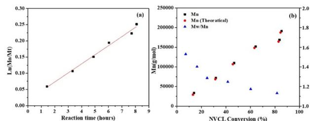
Fig. 4 (a) Semilogarithmic kinetic plot of consumption of monomer versus polymerization time. (b) Changes in  $\mathcal{D}$  ( $M_w/M_n$ ) and  $M_n$  of NVCL side chains with respect to monomer conversion.
