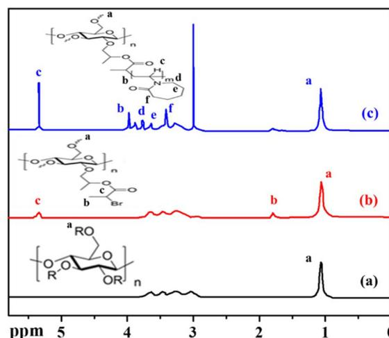
Fig. 2 <sup>1</sup>H NMR spectra of (a) HPC, (b) HPC-1, and (c) PNVCN-g-HPC.
