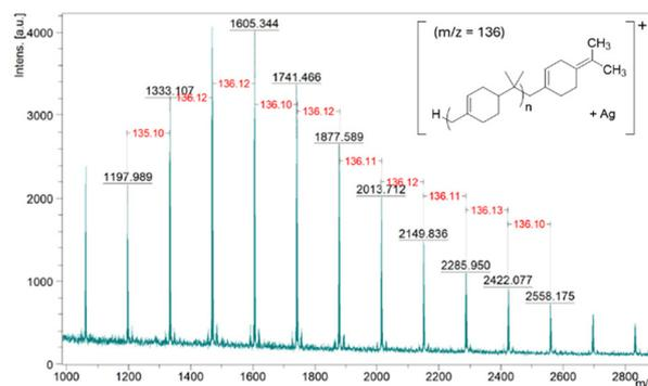
**Fig. 3** MALDI-ToF MS of PBP synthesised using  $\text{FeCl}_3$  as a catalyst. Silver trifluoroacetate was used as a cationisation agent and DCTB as a matrix. The predominant *endo* end group is shown, however both the *exo* and *endo* end groups are likely to be present.
