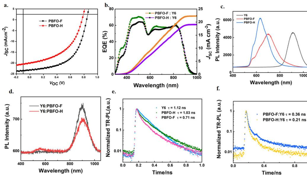
Fig. 3 (a)  $J$ – $V$  curves and (b) the corresponding EQE spectra of the OSCs based on the polymer:Y6 (c) PL spectra of Y6, PBFO-F and PBFO-H (d) PL spectra of Y6:PBFO-F and Y6:PBFO-H devices (e) TRPL spectra of Y6, PBFO-F and PBFO-H and (f) TRPL spectra of PBFO-F:Y6 and PBFO-H:Y6.
