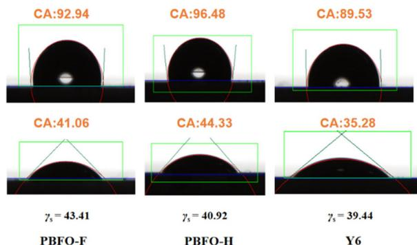
Fig. 5 Contact angles of PBFO-F, PBFO-H, and Y6 neat films with water and diiodomethane.
