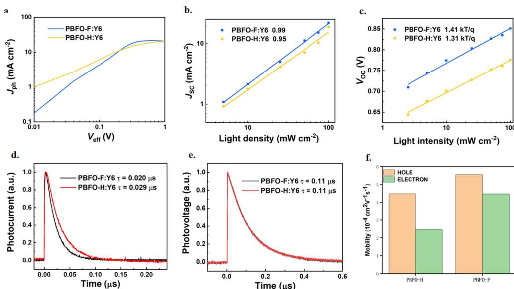
Fig. 4 (a) Photocurrent density ( $J_{ph}$ ) against effective voltage ( $V_{eff}$ ); dependence of (b)  $J_{SC}$  and (c)  $V_{OC}$  on  $P_{light}$  of the devices; (d) TPC curves; (e) TPV curves; and (f) charge mobility histogram.
