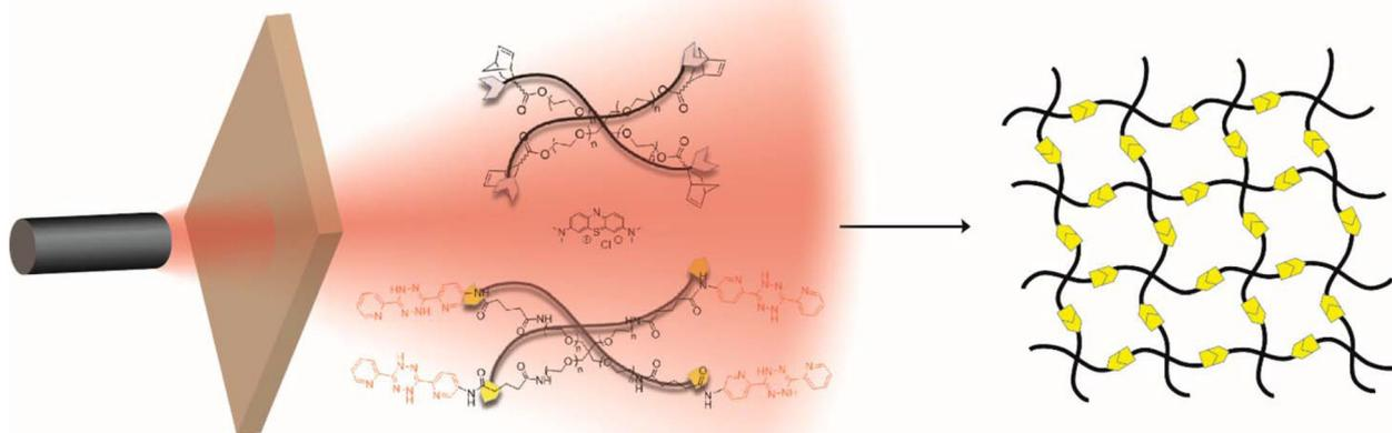
Fig. 8 The schematic illustration of hydrogel fabrication using red-light catalyzed Tz-IEDDA reaction. Adapted with permission from Truong *et al.*<sup>116</sup> Copyright © 2017, American Chemical Society.
