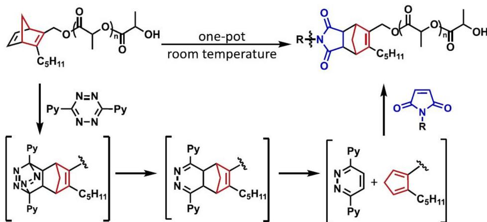
Fig. 6 One-pot functionalization of norbornadiene end-functional polymer with maleimides. Adapted with permission from Amant *et al.*<sup>71</sup> Copyright © 2019, American Chemical Society.
