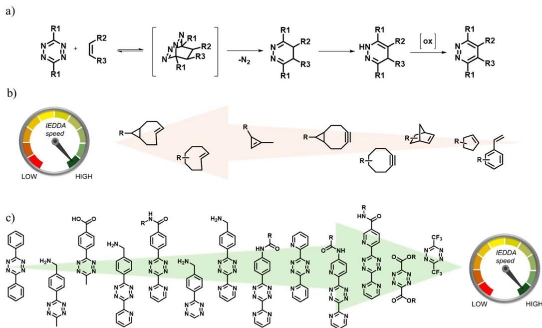
**Fig. 1** (a) The IEDDA cycloaddition reaction, (b) commonly employed dienophiles,<sup>1</sup> and (c) typical examples of Tz-based dienes.<sup>1</sup> Adapted with permission from Knall *et al.*<sup>1</sup> Copyright © The Royal Society of Chemistry 2013.
