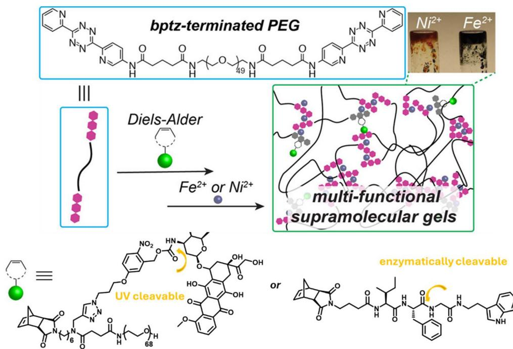
**Fig. 10** The schematic illustration of metallo-hydrogel using IEDDA reaction and metal coordination. Adapted with permission from Kawamoto *et al.*<sup>123</sup> Copyright © 2015, American Chemical Society.
