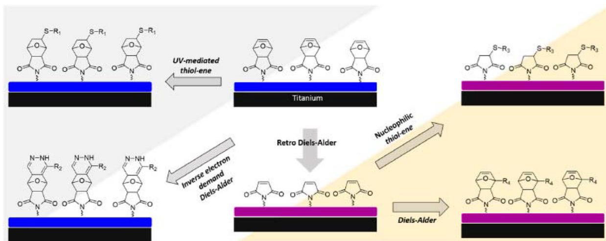
Fig. 17 Multi-functionalization of titanium surface bound hydrogels using different “click” chemistry reactions, including the IEDDA reaction. Adapted with permission from Gevrek et al.<sup>178</sup> Copyright © 2020, Molecular Diversity Preservation International (MDPI).
