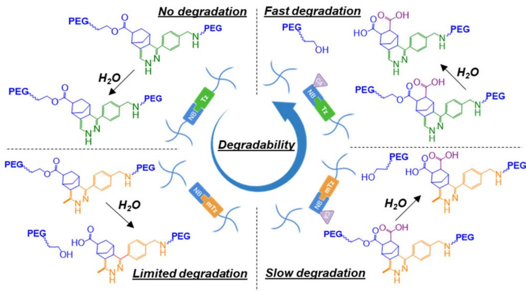
Fig. 9 Hydrolytic degradation of PEG-based Tz-IEDDA “click” hydrogels. Adapted with permission from Dimmitt *et al.*<sup>121</sup> Copyright © 2022, American Chemical Society.
