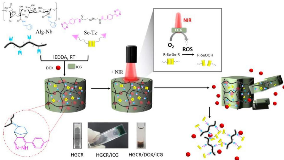
Fig. 15 Fabrication of Tz-IEDDA generated NIR-responsive alginate hydrogels. Adapted with permission from Anugrah et al.<sup>160</sup> Copyright © 2019, Elsevier.
