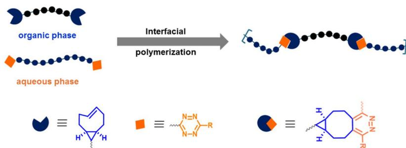
Fig. 3 Synthesis of multiblock copolymer fibers through interfacial bioorthogonal polymerization.<sup>34</sup>
