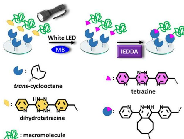
Fig. 16 Schematic illustration of a surface grafting approach based on light-induced inverse electron demand Diels-Alder (photo-IEDDA) reaction. Adapted with permission from Ozbek *et al.*<sup>175</sup> Copyright © 2021 American Chemical Society.
