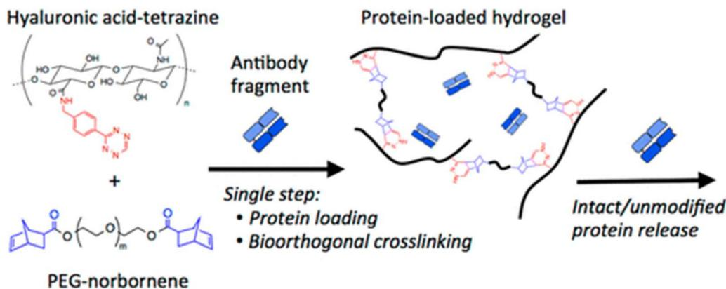
Fig. 12 Schematic illustration of fabricating protein-releasing hydrogels using Tz-IEDDA-based crosslinking of hyaluronic acid and PEG polymers. Adapted with permission from Famili *et al.*<sup>138</sup> Copyright © 2017, American Chemical Society.
