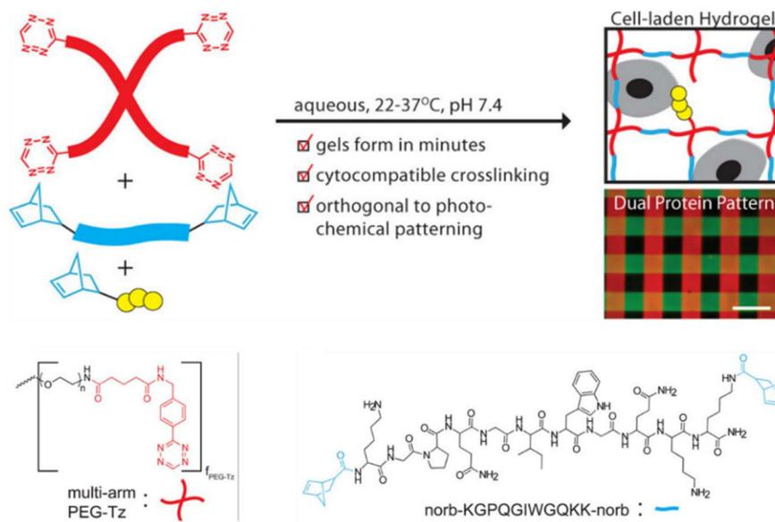
**Fig. 11** Overview of hydrogel formation by Tz-NB IEDDA reaction using multi-functional PEG-Tz and cell degradable dinorbornene crosslinker peptide. Adapted with permission from Alge *et al.*<sup>125</sup> Copyright © 2013, American Chemical Society.
