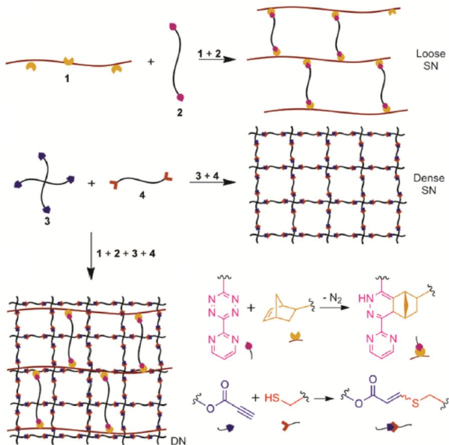
Fig. 7 Schematic of double network hydrogel formation via dual "click" approach. Adapted with permission from Truong *et al.*<sup>112</sup> Copyright © 2015, American Chemical Society.
