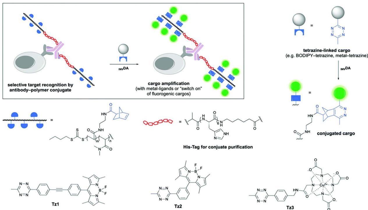
Fig. 5 Preparation of Tz-IEDDA reaction-mediated polymer-protein conjugates for fluorescent signal amplification. Adapted with permission from Zhang *et al.*<sup>66</sup> Copyright © 2020, The Royal Society of Chemistry.
