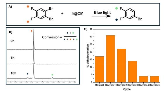
Fig. 7 (A) Reaction scheme of dehalogenation; (B) <sup>19</sup>F NMR of reaction mixture at different time points. Debromination is indicated by the appearance of two peaks at –135.25 ppm and –139.75 ppm. (C) Dehalogenation efficiency of pbtz-Ir@CM over numerous cycles determined by integration of peaks at –135.25 ppm and –139.75 ppm against 1,2-dibromo-4,5-difluorobenzene peak at –136.4 ppm.
