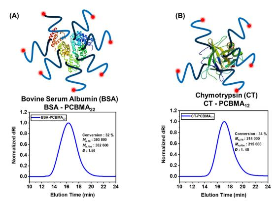
Fig. 4 Synthesis of protein-polymer hybrids (PPH) by heterogenous CM-EY catalyzed photo-ATRP (A) BSA-PCBMA22 and (B) CT-PCBMA12. Reaction conditions: ([CBMA]/[Proetin-I]/[CM-EY]/[CuBr<sub>2</sub>]/[TPMA]/[TEOA]) = 200/1/0.005/0.2/0.6/0.6 in 1x PBS under green light irradiation  $(525 \text{ nm}, 25 \text{ mW cm}^{-2}), \text{CM-EY} = 1.6 \text{ mg mL}^{-1}.$
