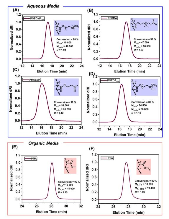
Fig. 3 Expanding monomer scope of heterogenous CM-EY catalyzed photo ATRP to (A) POEOMA<sub>300</sub>, (B) PCBMA, (C) PMSEMA, (D) POEOA<sub>480</sub>, (E) PMA and (F) PEA.
