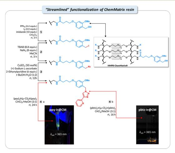
Fig. 6 Synthesis of ppy-lr@CM and pbtz-lr@CM via the "streamlined" functionalization of ChemMatrix. ppy = phenyl-pyridine, pbtz = 2-(4-(trifluoromethyl)phenyl)benzo[d]thiazole, TBAB = tetrabutylammonium bromide.
