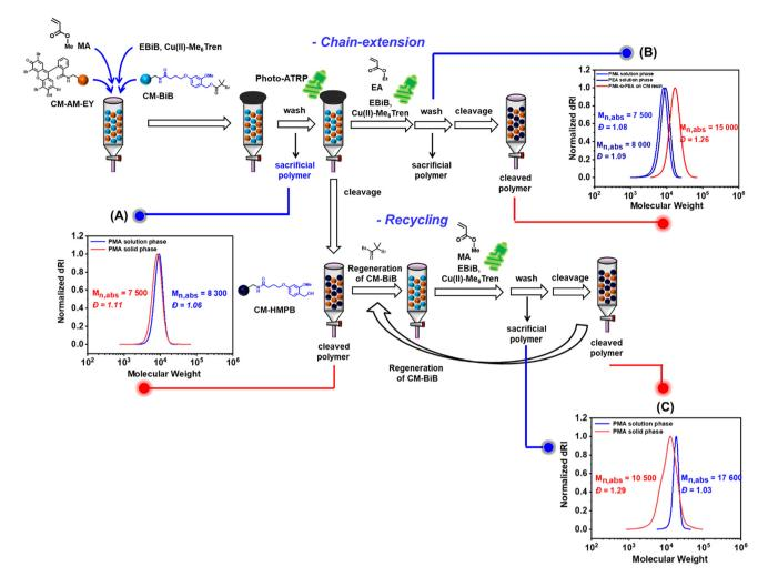
Fig. 5 (A) Solid-phase synthesis of polymers catalyzed by heterogenous CM-AM-EY (A) homopolymer of PMA grafted from CM-BIB, (B) block copolymer of PMA-b-PEA grafted from CM-BIB and (C) recycling of CM-BIB and CM-AM-EY for solid-phase polymer synthesis.
