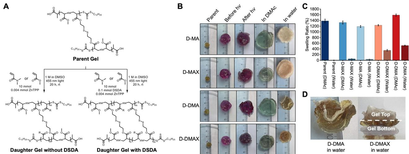
**Fig. 3** (A) Scheme of parent-to-daughter gel network extension. (B) Photographs of the dried parent networks, parent networks swelled before irradiation, parent networks after irradiation to synthesize daughter gels, daughter gels swelled in DMAc, and daughter gels swelled in water. (C) Swelling ratios of parent and daughter gels in DMAc and water. (D) Photographs of the side profiles of D-DMA and D-DMAX swelled in water with designations for the top and bottom of the daughter gels.
