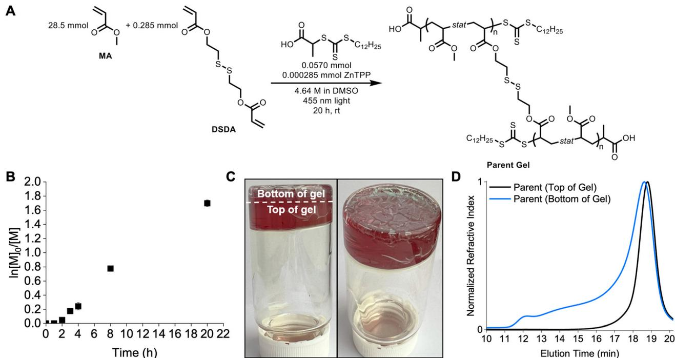
**Fig. 2** (A) Scheme of parent gel polymerization. (B) Pseudo-first-order kinetic plot of the parent gel polymerization. (C) Photographs of the resulting parent gel following irradiation. (D) SEC traces of the parent gel with samples taken from the top and bottom of the gel.
