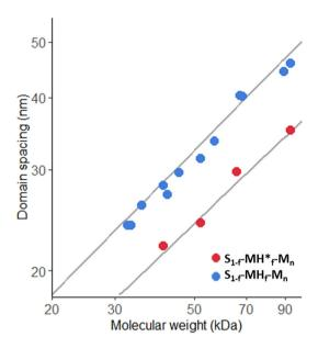
Fig. 4 Double logarithmic plot of the domain spacing against the molecular weight for the lamellar morphology determined from  $d_{SAXS}$ The dark grey lines are the power law fits to  $d = a*MW^b$ .
