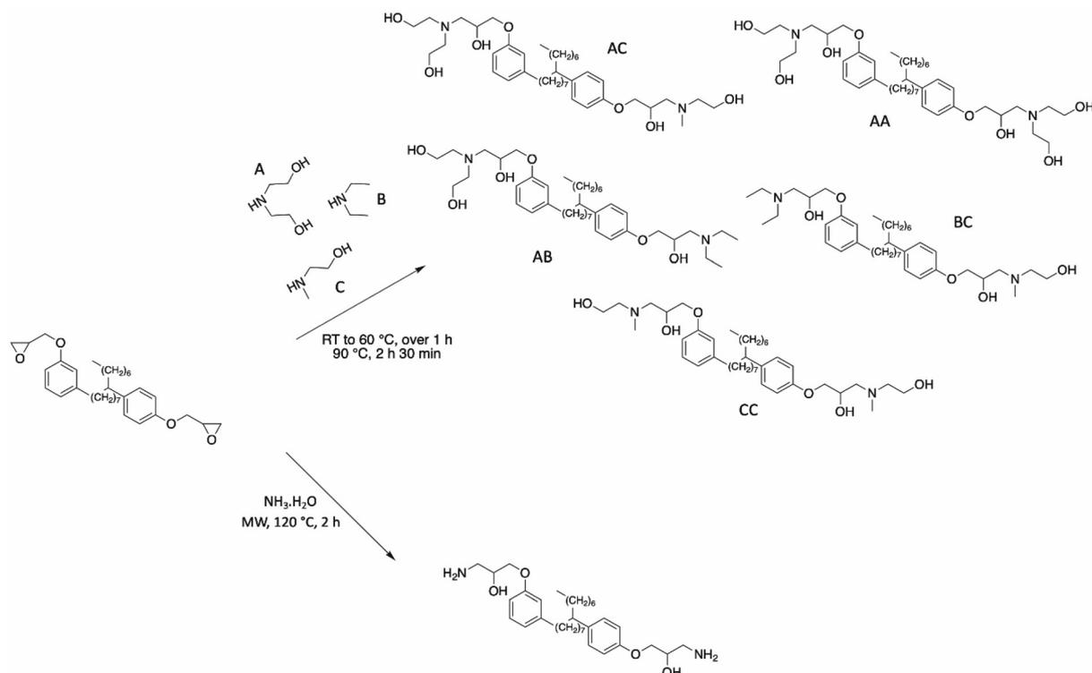
**Scheme 14** Synthesis of various polyols based on commercial NC-514 by Kathalewar *et al.*<sup>100</sup> and Mora *et al.*<sup>80</sup>
