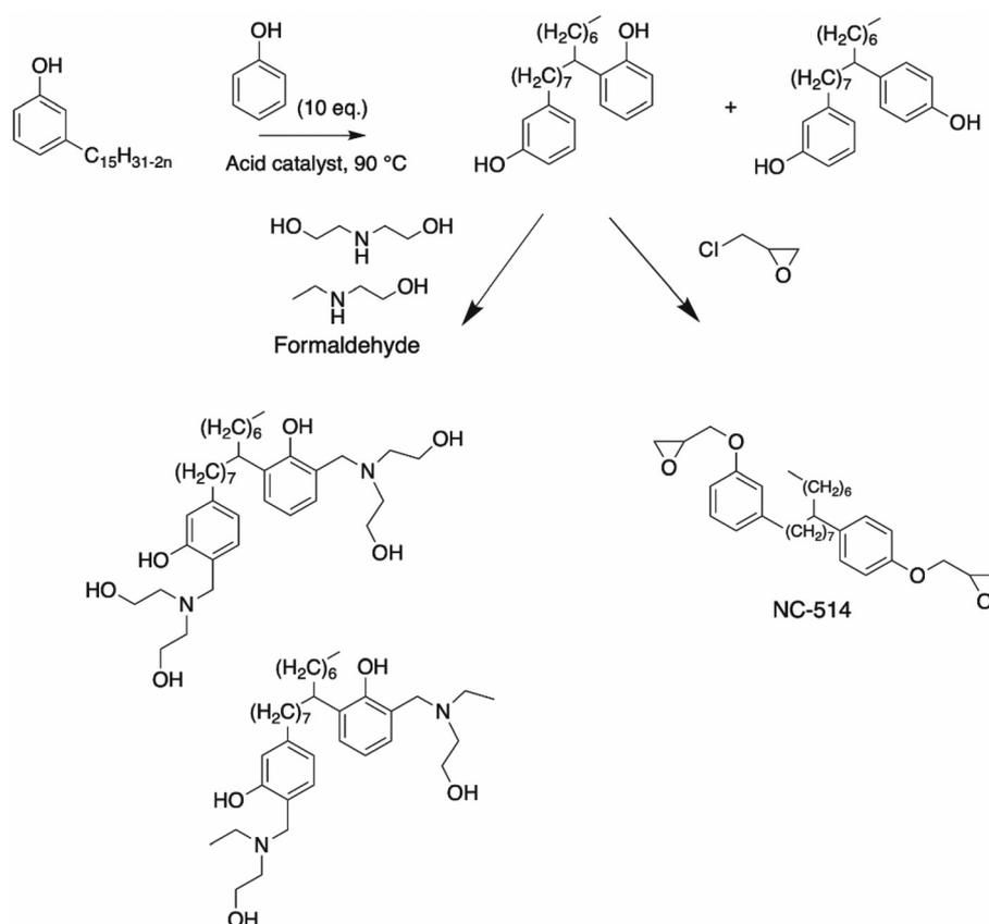
**Scheme 13** Synthesis of bisphenol cardanol through alkyl chain unsaturation by Ramasri *et al.*,<sup>96</sup> and the formation of a polyol by Ramasri *et al.*<sup>99</sup> and NC-514 molecule.
