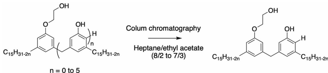
Scheme 24 Separation of Cardolite resin for the preparation of cardanol-based dimer.<sup>120</sup>
