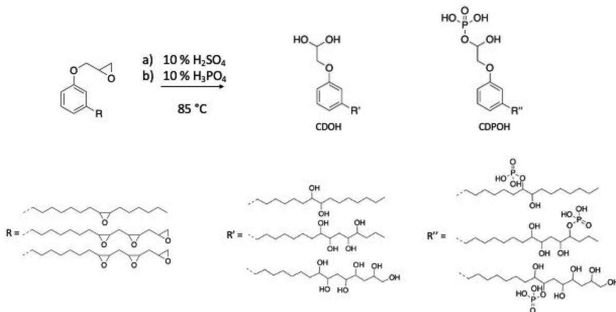
Scheme 5 Hydrolysis reaction to open epoxy ring by Somiseti *et al.*<sup>1</sup>
