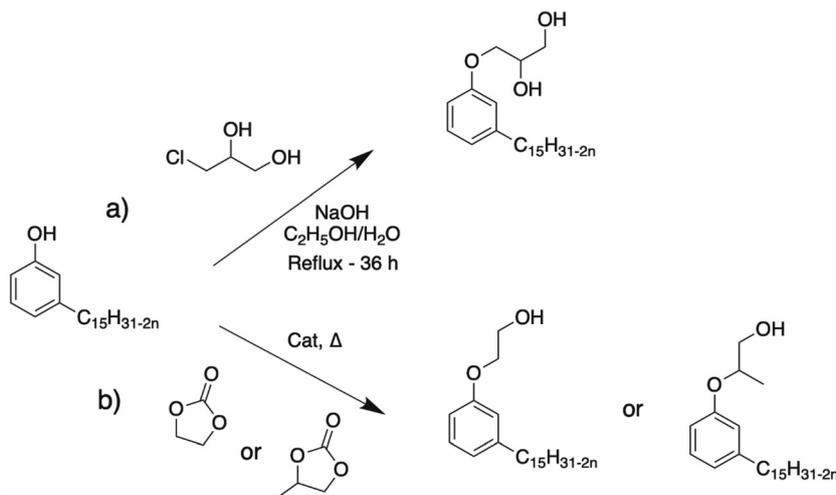
**Scheme 2** Synthetic pathway for the etherification of cardanol to form (a) diol<sup>73</sup> and (b) alcohol.<sup>74</sup>
