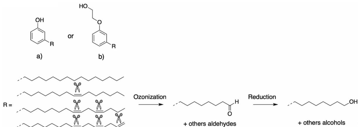
Scheme 12 Oxidative cleavage of the unsaturated alkyl chain of cardanol by Tyman *et al.* and Dinon *et al.*<sup>92,93,95</sup>
