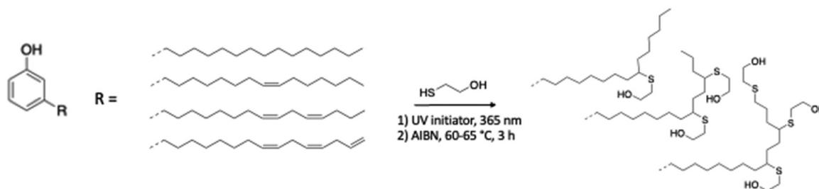
**Scheme 10** Thiol-ene coupling on unsaturation of cardanol alkyl chains using a (1) photochemical initiator by Fu *et al.*<sup>89</sup> or (2) thermal initiator by Shrestha *et al.*<sup>90</sup>
