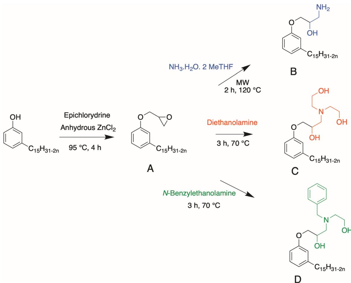
**Scheme 3** Synthesis pathways of epoxidation of cardanol and epoxy ring opening to obtain cardanol-based polyols.<sup>78–82</sup>
