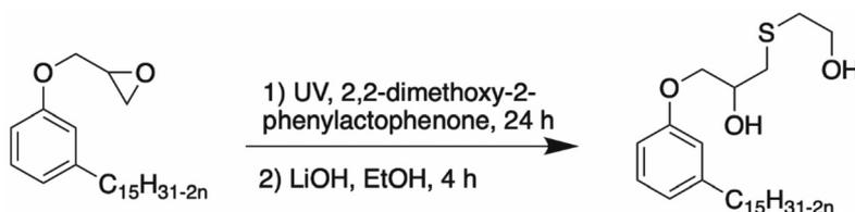
**Scheme 4** Epoxy ring opening of a cardanol derivative by a thiol by Wang *et al.*<sup>83</sup>
