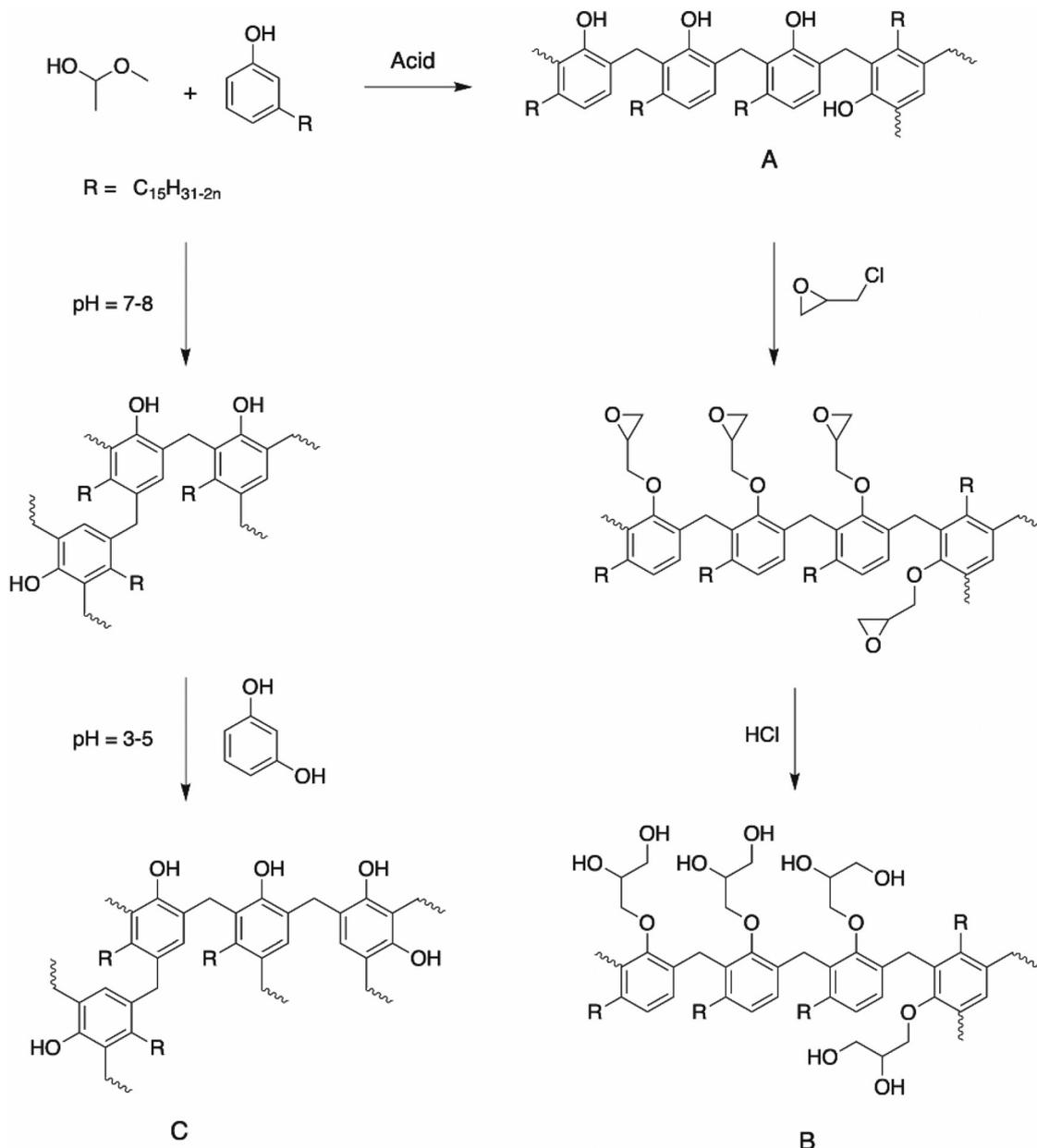
**Scheme 26** Polyols from cardanol-based novolac resins synthesized by (A) Mythili *et al.*,<sup>124</sup> (B) Sathiyalekshmi *et al.*<sup>125,126</sup> and (C) Mahajan *et al.*<sup>35</sup>
