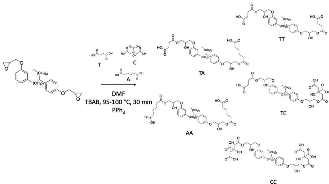
**Scheme 15** NC-514 modified with bio-based acid to form novel cardanol-based polyols.<sup>101,102</sup>
