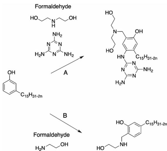
**Scheme 20** Synthesis of Mannich-based polyol by Zhang *et al.*<sup>114</sup> (A) and Oh *et al.*<sup>115</sup> (B).
