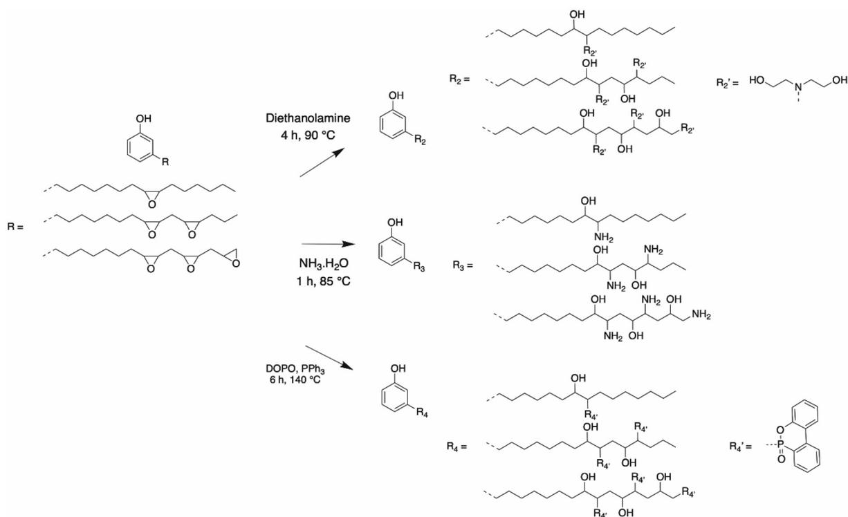
**Scheme 8** Amination of the epoxy ring by Huo<sup>81</sup> and Mora *et al.*<sup>80</sup> and phosphorylation by Bo *et al.*<sup>87</sup>
