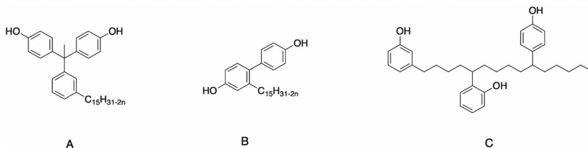
Fig. 5 Structure of cardanol-based bisphenol used in (A) polycondensation of PEEK by More *et al.*,<sup>178</sup> (B) polycondensation of poly(arylene ether) by Tawade *et al.*<sup>179</sup> and (C) phenolic foam by Jing *et al.*<sup>97</sup>
