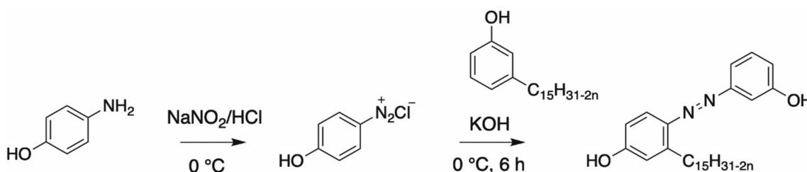
**Scheme 17** Synthesis of azo cardanol-based polyol by Bhunia *et al.*<sup>105–107</sup>
