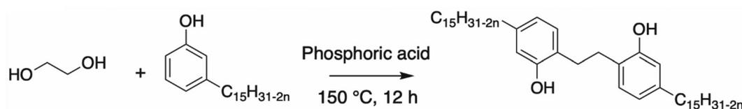
Scheme 22 Dimerization of cardanol by Tan *et al.*<sup>117</sup>
