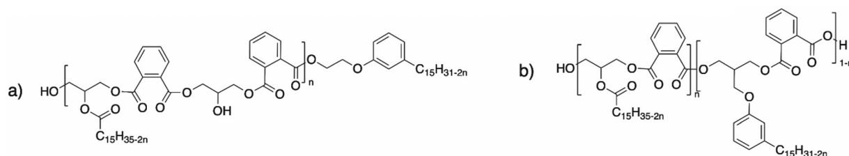
**Scheme 33** Structures of alkyd resins with (a) monofunctional hydroxyl cardanol and (b) difunctional hydroxyl cardanol by Denis *et al.*<sup>175</sup>
