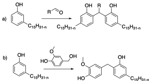
**Scheme 25** Synthesis of cardanol dimers from (a) controlled condensation with aldehydes<sup>121,122</sup> and (b) condensation with vanillyl alcohol.<sup>123</sup>
