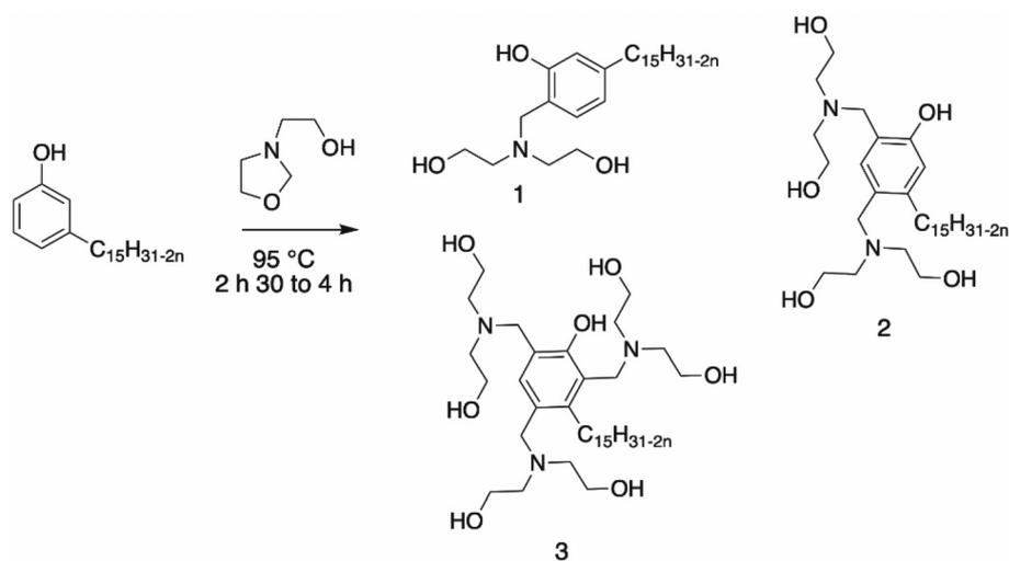
**Scheme 19** Synthesis of Mannich-based polyol by Ionescu *et al.*<sup>113</sup> and Asif *et al.*<sup>112</sup>
