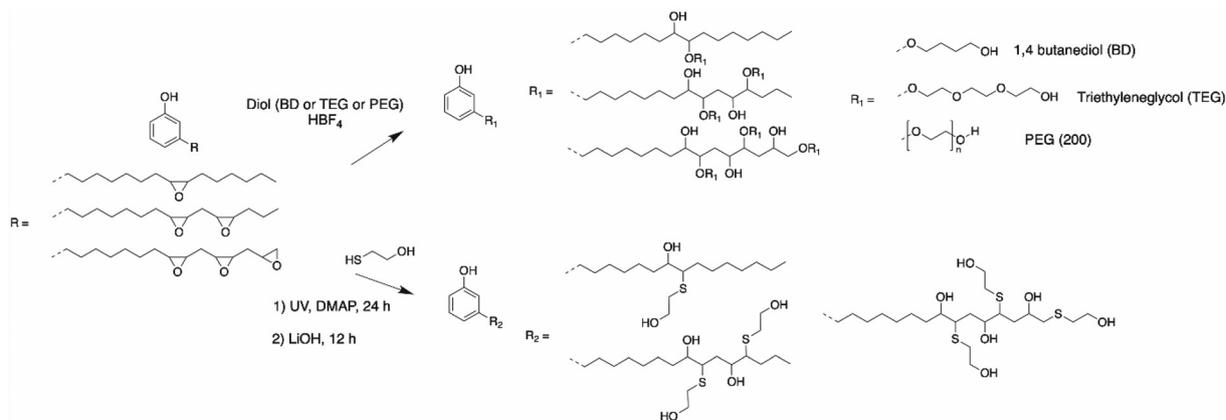
**Scheme 9** Formation of polyol cardanol through etherification of epoxy ring by Kim *et al.*<sup>88</sup> and addition of functionalized thiol on the epoxy ring by Wang *et al.*<sup>83</sup>
