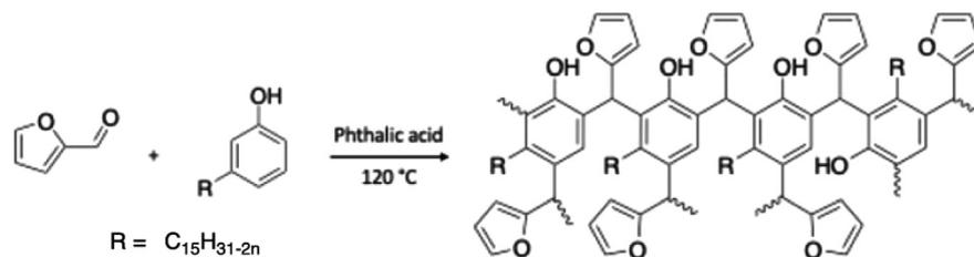
**Scheme 27** Polyol-based cardanol furfural resin by Joy *et al.*<sup>127</sup>
