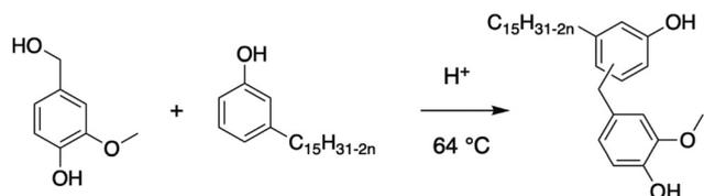
**Scheme 16** Condensation of vanillyl alcohol and cardanol to form cardanol-based polyol by Basset *et al.*<sup>104</sup>
