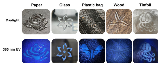
Fig. 5 Fluorescent patterns of PUHG adhering to paper, glass, plastic, wood and tinfoil under daylight and an ultraviolet lamp.
