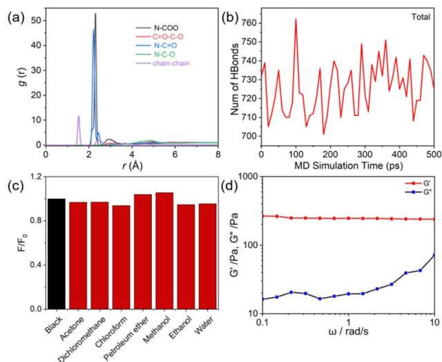
**Fig. 4** (a) Radial distribution function of **PUHG** by molecular dynamics simulation. (b) The number of total hydrogen bonds over time. (c) Fluorescence changes of pure **PUHG** (black) and **PUHG** treated with different solvents (red). (d) The elastic modulus ( $G'$ ) and viscosity modulus ( $G''$ ) at different frequencies of **PUHG**.
