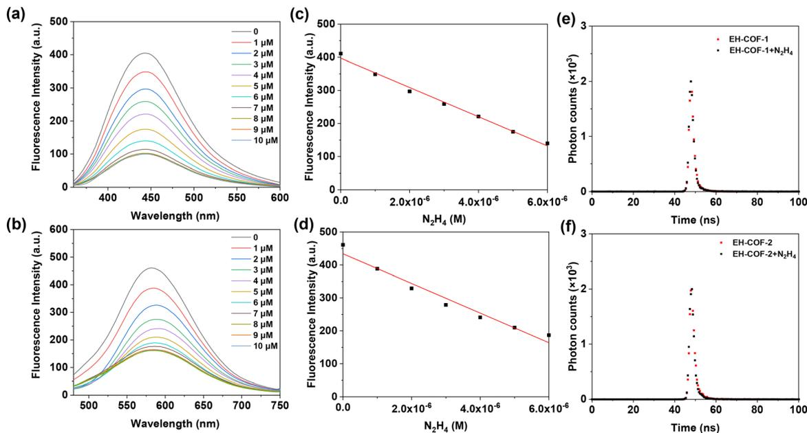
**Fig. 5** Fluorescence spectra of (a) EH-COF-1 and (b) EH-COF-2 with different concentration of hydrazine. Fluorescence intensity of (c) EH-COF-1 and (d) EH-COF-2 with different concentration of hydrazine. Lifetimes of (e) EH-COF-1 and (f) EH-COF-2 with and without hydrazine.
