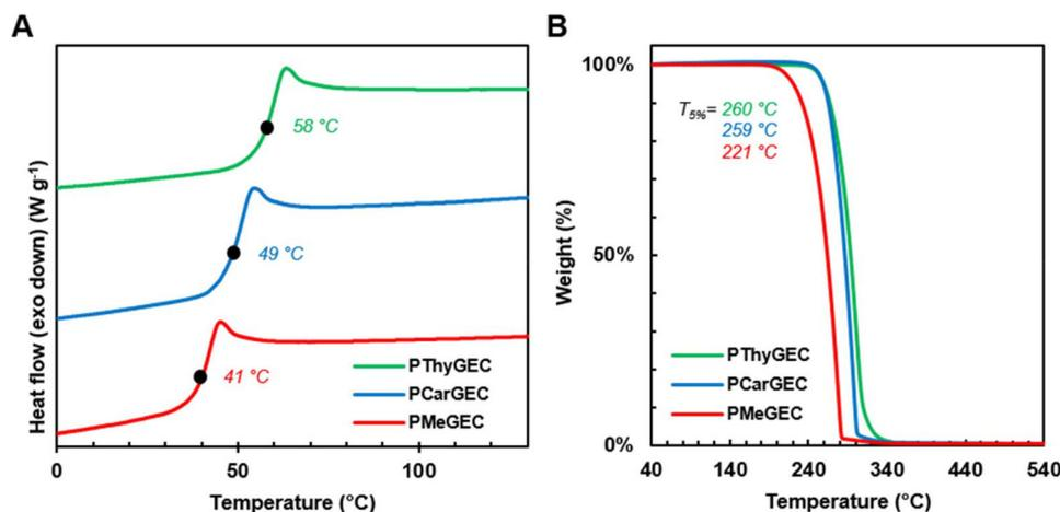
Fig. 3 (A) DSC measurements and (B) TGA measurements of the three different terpenoid-based copolymers.
