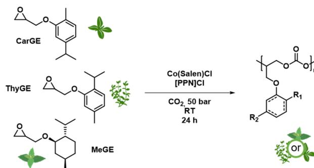
**Scheme 1** Synthesis of cyclic terpenoid-based polycarbonates.
