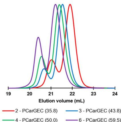
**Fig. 2** SEC traces of PCarGEC presented in Table 1 with different catalyst loading ratios (THF, PS, RI detector). M<sub>n</sub> of the respective polymers is shown in the legend.
