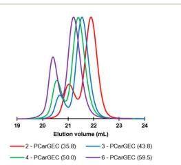
Fig. 2 SEC traces of PCarGEC presented in Table 1 with different catalyst loading ratios (THF, PS, RI detector).  $M_n$  of the respective polymers is shown in the legend.
