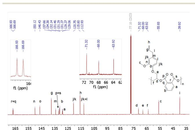
**Fig. 4**  $^{13}\text{C}\{^1\text{H}\}$  NMR spectrum (125 MHz,  $\text{CDCl}_3$ ) of isolated p(PA-*alt*-EGE) formed from the ROCOP of PA and EGE initiated by IPr. Conditions: 250/300/1 (PA/CHO/IPr), no solvent, 90 °C, 16 h (100% conversion of PA).
