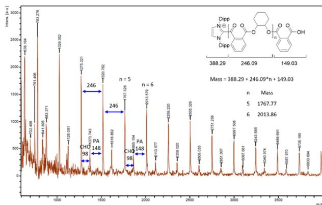
**Fig. 2** MALDI-TOF mass spectrum (zoom of a region) for isolated poly(PA-*alt*-CHO) formed from the ROCOP of PA and CHO initiated by IPr. Conditions: 60/70/1 (PA/CHO/IPr), no solvent, 90 °C, 16 h (95% conversion of PA). See the ESI† for the full MALDI-TOF spectrum.
