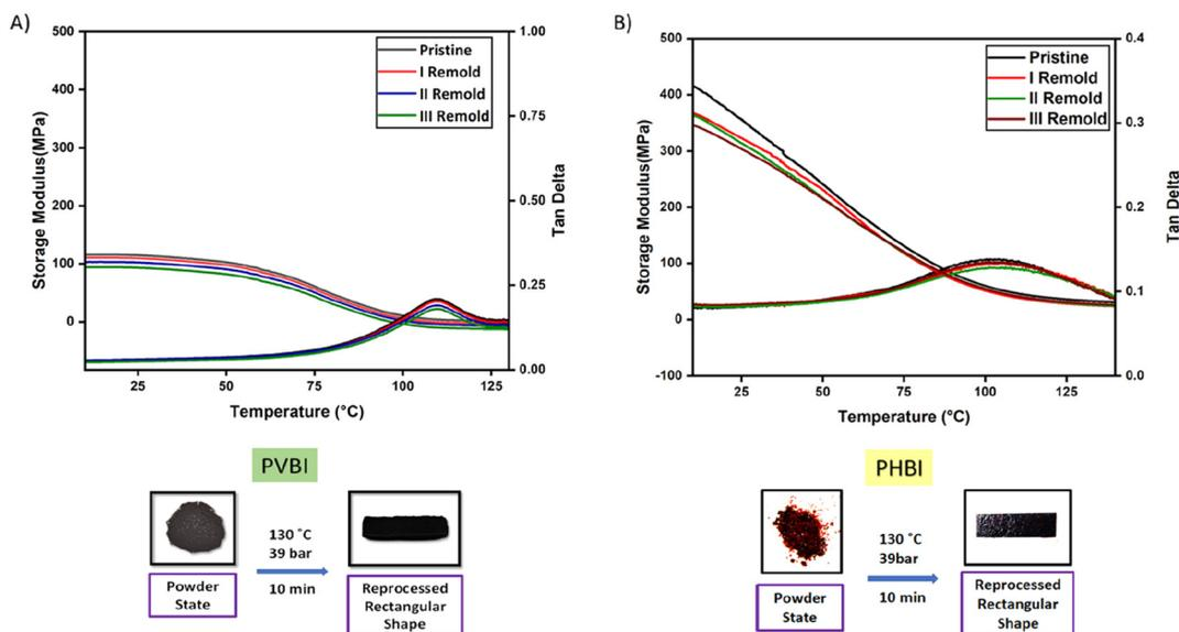
**Fig. 6** (A) Storage modulus and  $\tan \delta$  vs. temperature plots in PVBI along with reprocessing images and conditions and (B) Storage modulus and  $\tan \delta$  vs. temperature plots in PHBI along with reprocessing parameters used in hot-pressing.
