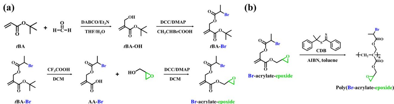
Scheme 2 Synthesis of (a) the Br-acrylate-epoxide functional monomer and (b) the poly(Br-acrylate-epoxide) macro-agent.
