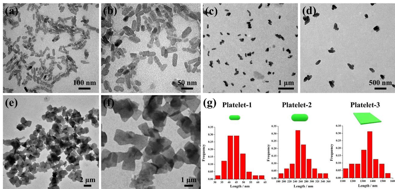
**Fig. 3** TEM images of 2D platelets formed by PA-g-PAzo/PEG/PLA in a mixture of CH<sub>3</sub>OH and THF ( $V_{\text{methanol}} : V_{\text{THF}} = 92 : 8$ ) with concentrations of (a, b) 0.015 mg mL<sup>-1</sup>, platelet-1, (c, d) 0.02 mg mL<sup>-1</sup>, platelet-2, and (e, f) 0.04 mg mL<sup>-1</sup>, platelet-3. (g) Statistical analysis of the length distribution of the platelets.
