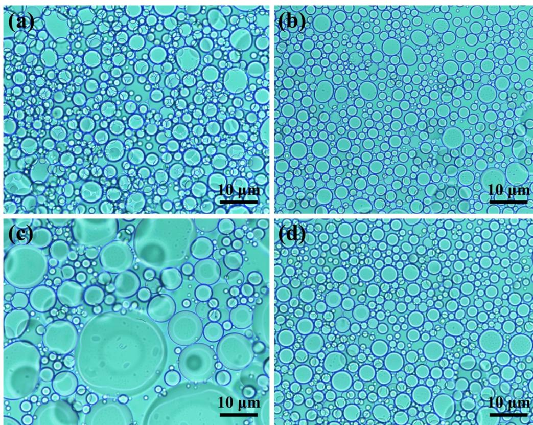
Fig. 6 Optical microscopy images of the emulsions prepared using hexafluorobenzene as the oil phase: PEG-*b*-PFA as the surfactant after storing for (a) 24 h and (c) 7 d, and PA-*g*-PFA/PEG/PLA as the surfactant after storing for (b) 24 h and (d) 7 d.
