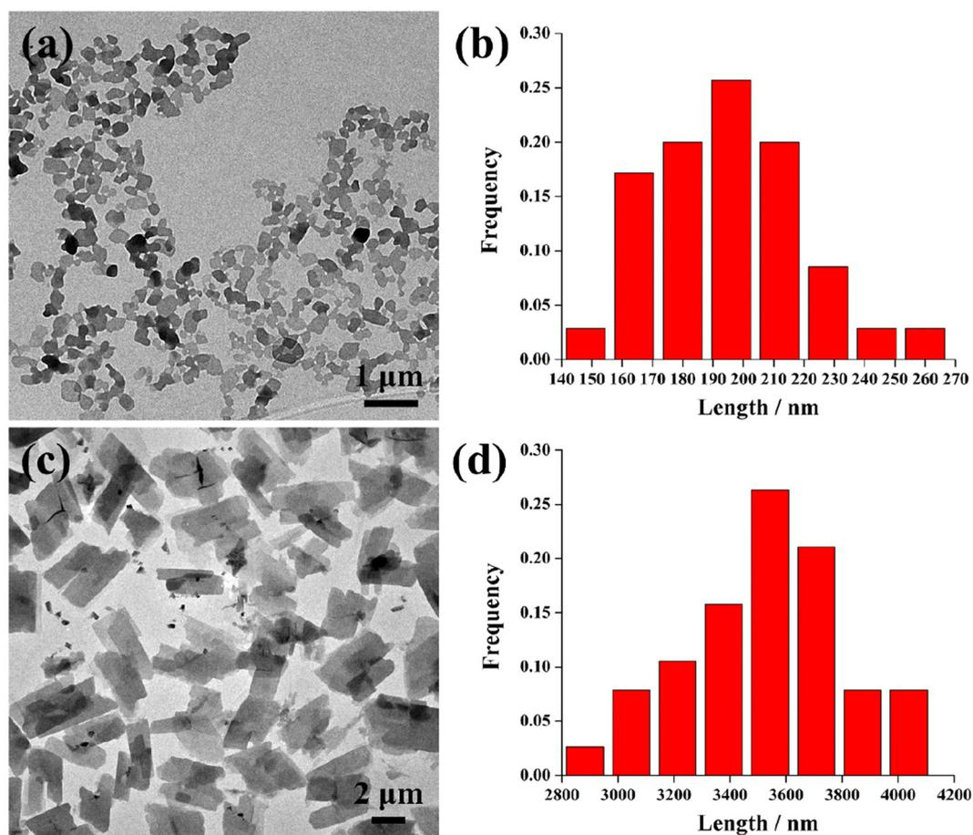
**Fig. 4** TEM images of 2D platelets formed by PA-g-PAzo/PEG/PLA in a mixture of CH<sub>3</sub>OH and THF ( $V_{\text{methanol}} : V_{\text{THF}} = 95 : 5$ ) with concentrations of (a) 0.01 mg mL<sup>-1</sup> and (b) 0.05 mg mL<sup>-1</sup>.
