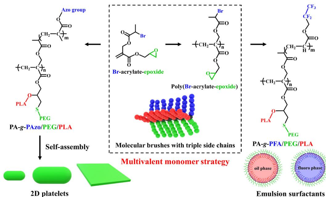
**Scheme 1** Chemical structures of the multivalent monomer Br-acrylate-epoxide, the macro-agent poly(Br-acrylate-epoxide), and the asymmetric molecular brushes with triple side chains PA-*g*-PAzo/PEG/PLA and PA-*g*-PFA/PEG/PLA. Schematic representations of the self-assembly behavior of PA-*g*-PAzo/PEG/PLA and the surfactant properties of PA-*g*-PFA/PEG/PLA.
