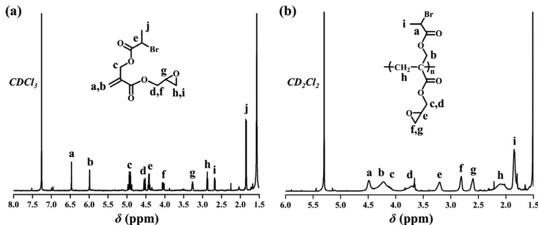
Fig. 1 <sup>1</sup>H NMR spectra of (a) the Br-acrylate-epoxide functional monomer and (b) the poly(Br-acrylate-epoxide) macro-agent.
