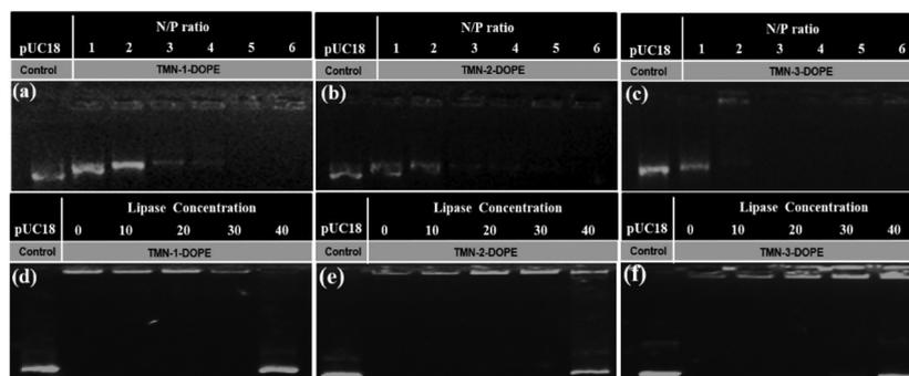
**Fig. 2** Agarose gel electrophoresis of pUC18 DNA complexed with polymers TMN-1/2/3-DOPE at different N/P ratios in 20 mM Tris-HCl buffer (a–c). Agarose gel electrophoresis of the dissociation of condensed DNA at different concentrations of lipase [TMN-1-DOPE: N/P = 5, TMN-2-DOPE: N/P = 5, TMN-3-DOPE: N/P = 3] (d–f). [pUC18 DNA] = 9  $\mu\text{g mL}^{-1}$ , [lipase] = 10–40  $\mu\text{g mL}^{-1}$ , 37  $^{\circ}\text{C}$ .
